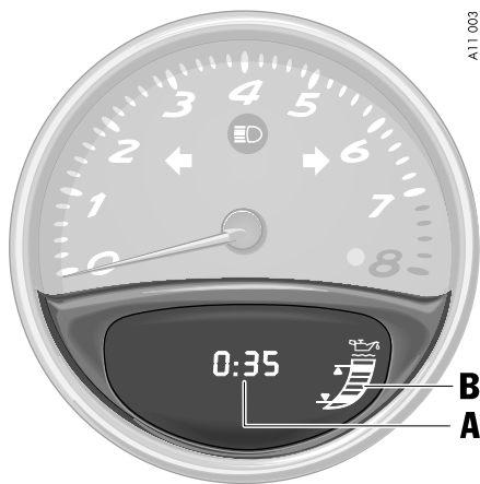
A - Waiting time display for oil level measurement B - Engine oil level segment display
