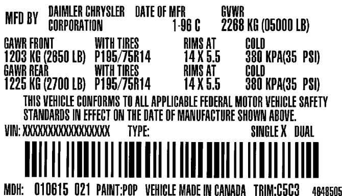
Fig. 1 VEHICLE SAFETY CERTIFICATION LABEL - TYPICAL
