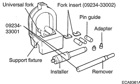
2. The piston pin is press fit into the rod little end, and the piston floats on the pin.
