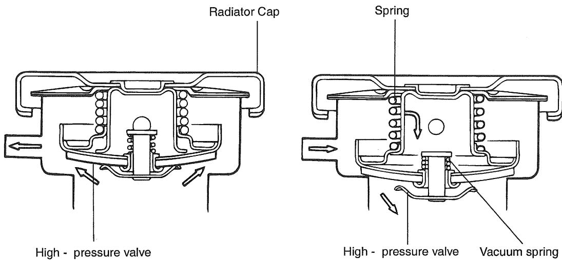
When the pressure is reduced to the specified level
