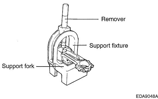
5. To install a new pin, the proper fork inserts must be in place to support the rod.
