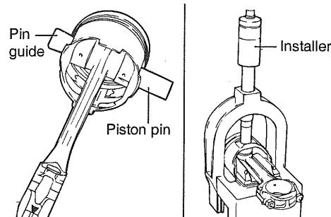
7. Insert the installer tool through the hole in the arch of the support fixture and use a hydraulic press to force the piston pin through the rod little end. Continue pressing until the pin guide falls free and the installer tool seats against the top of the arch.
