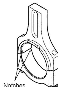
1. Remove the connecting rod cap bolts, then remove the caps and the big end lower bearing.
