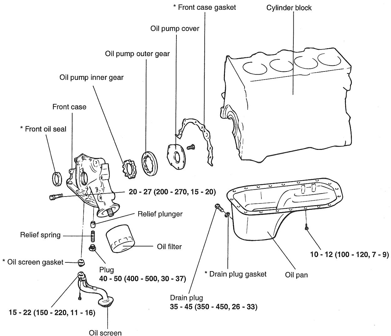
\* Replace the gasket and seal with new ones after removal.
