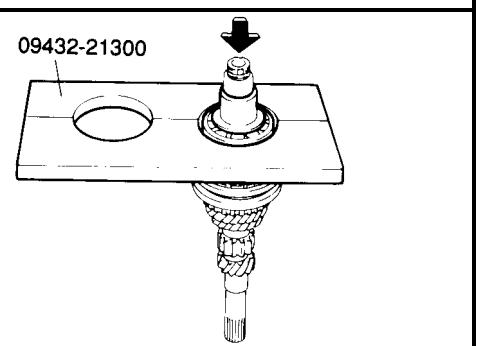
6. Remove the fourth speed gear and needle roller bearing, synchro nizer ring, third-fourth speed synchronizer sleeve.
