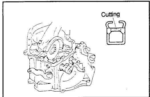
4. Grind the head of lock pin and shifting control shaft over 5mm.
