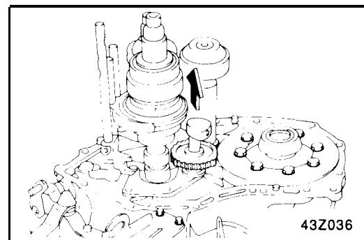
18. Remove the spring pins using the special tool (09414-11000).
