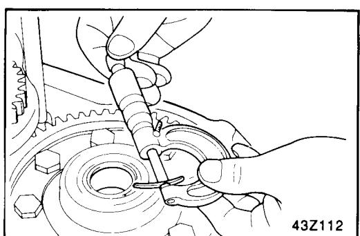
19. Install the oil guide to the transaxle case.
