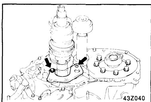
21. Lift up the input shaft assembly and remove the intermediate shaft assembly.
