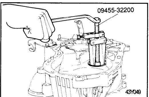
25. Remove the differential bearing oil seal and the differential bearing outer race.
