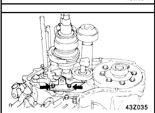
17. Remove the reverse gear shaft and reverse gear.
