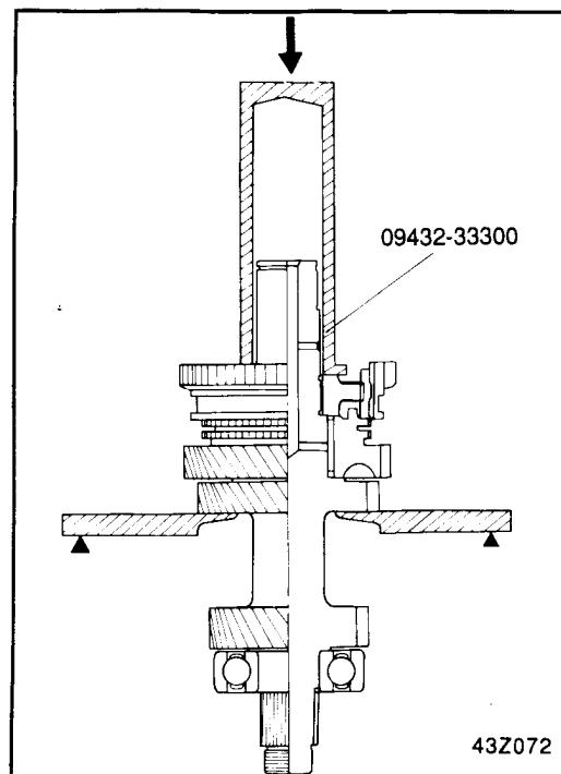
7. Install the needle roller bearing, first speed gear, bearing sleeve together using the special tool (09432-33300).
