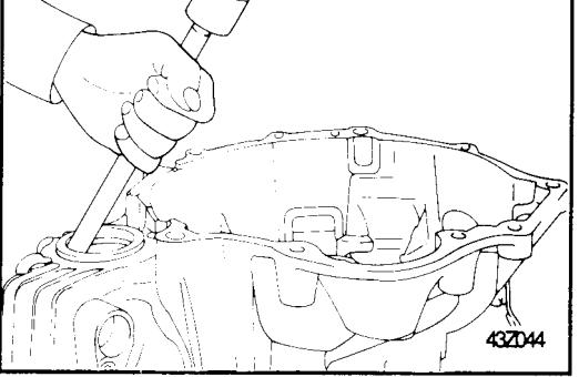
26. Remove the input shaft oil seal.
