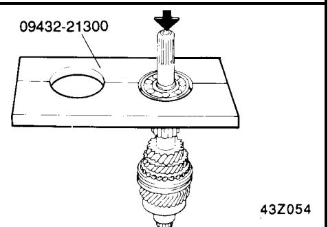
3. Remove the bearing sleeve using the special tool (09455-21000).
