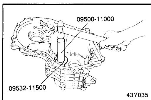
16. Install the differential bearing outer race and spacer to the transaxle case using the special tools (09500-11000, 09532-11500).
