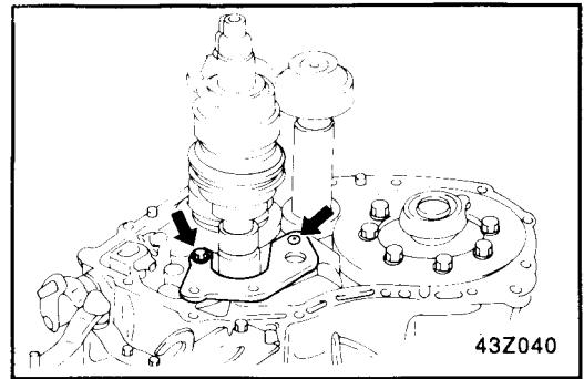
9. Reassembly of shift rail assembly.
