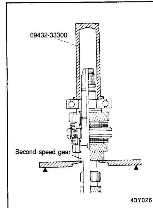
10. Install the rear bearing sleeve using the special tool (09432-33300).
