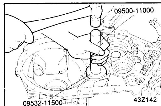
5. Install the oil guide and intermediate shaft bearing outer race and spacer using the special tools (09500-21000, 09432-33400).
