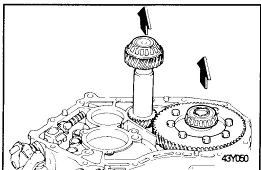
23. Remove the intermediate shaft bearing outer race and spacer and oil guide using the special tool (09455-32200).
