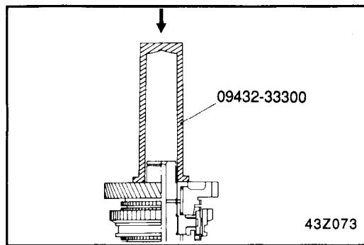
8. Install the taper bearing using the special tool (09432-33300).
