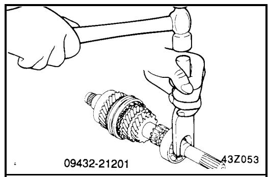
2. Remove the front bearing using the special tool (09432-21300).
