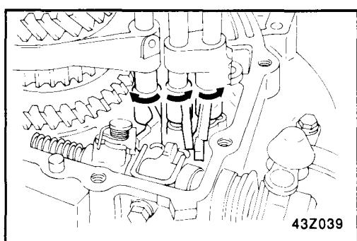
20. Remove the bearing retainer.
