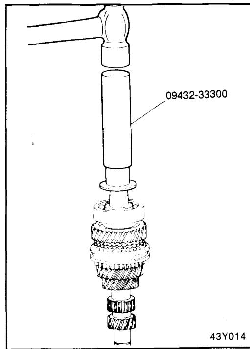
11. Install the front bearing using the special tool (09432-33300).
