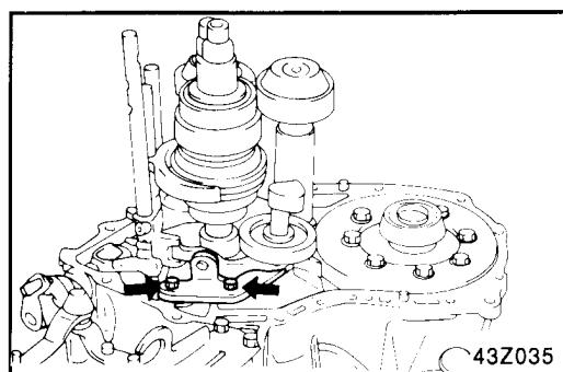
14. Install the intermediate shaft bearing outer race and spacer to the transaxle case using the special tools (09500-21000, 09432-33400).
