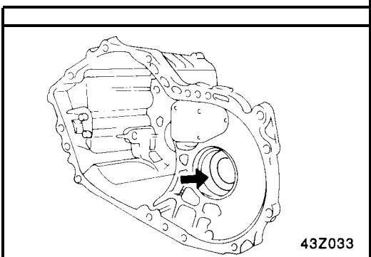
13. Remove the output shaft bearing outer race and spacer using the special tool (09455-32200).
