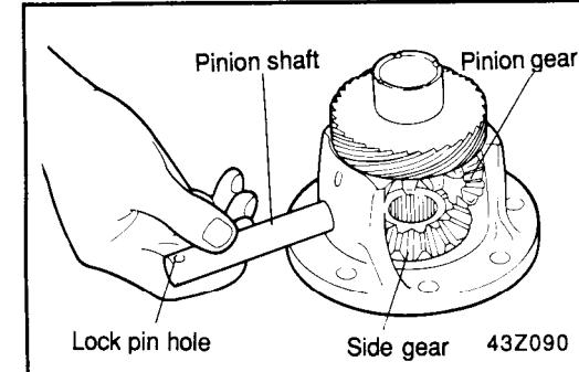
4. Measure the backlash between the side gears and pinions.
