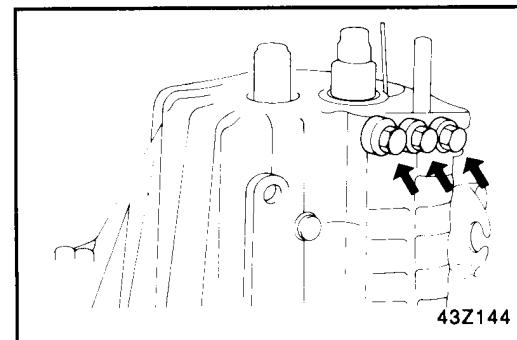
27. Install the intermediate gear using the special tool (09432-33300).
