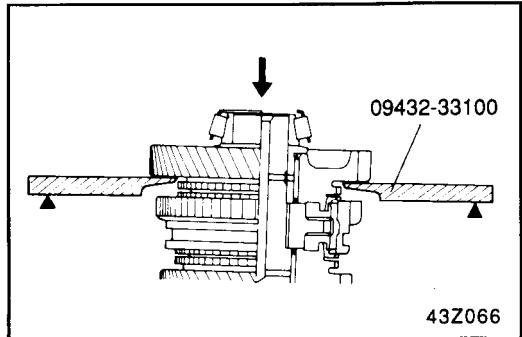
3. Remove the first-second speed synchronizer assembly and second speed gear, needle roller bearing together using the special tool (09432-33100).
