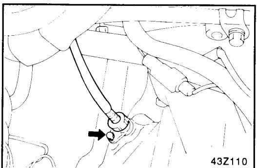
7. Remove the starter motor mounting bolts.
