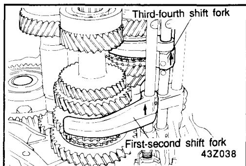
3) Remove the shift rail assembly.
