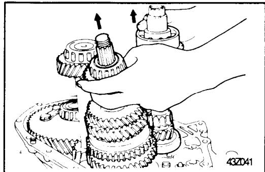
22. Remove the output shaft assembly and differential gear assembly.
