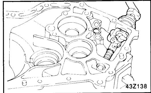
4. Install new spring pins using the special tool (09414-11100).
