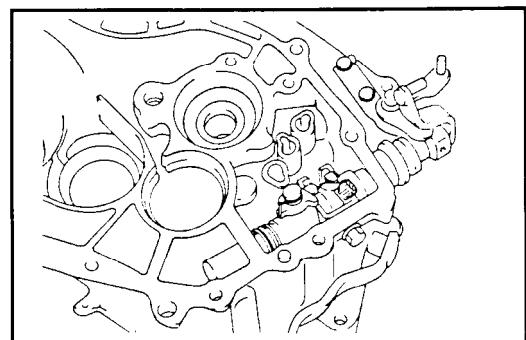
6. Remove the lock pin from the shifting control shift by punching the bottom of the lock pin using the special tool (09414-11000).
