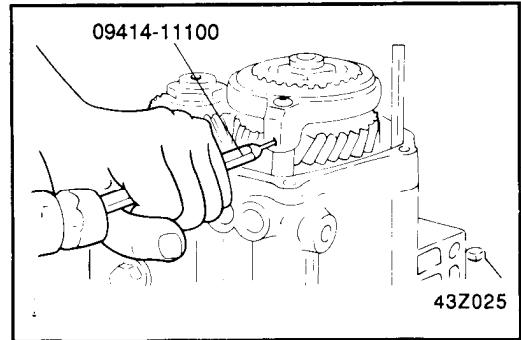
31. When installing, make sure that the slit of the spring pin is aligned with the shift railcenter line.
