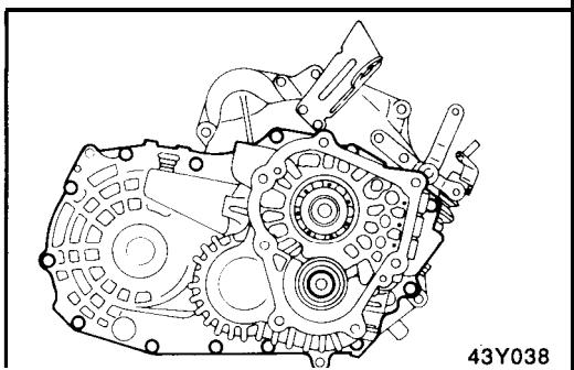
12. Remove the differential oil seal and oil guide.
