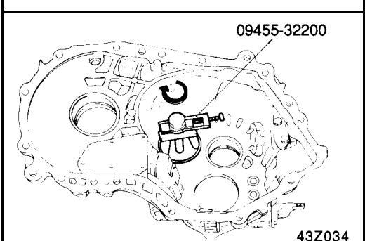
16. Remove the reverse shift lever and the reverse shift shoe.
