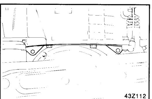
11. Remove the transaxle assembly lower mounting bolts with the transaxle assembly supported by a jack.
