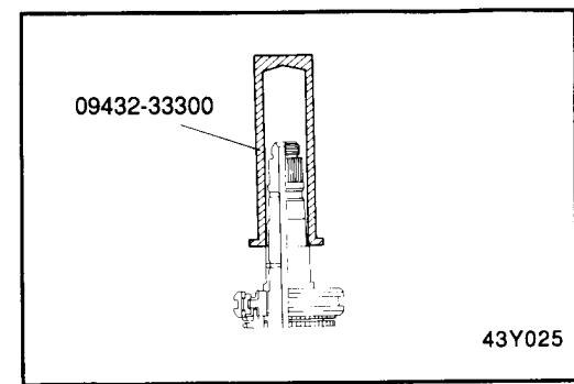
8. Install the rear bearing using the special tool (09432-33300).
