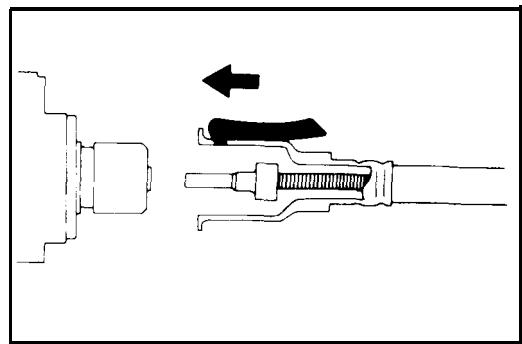
3. Install the grommet so that, as shown in the illustration, the cable attachment part and the projecting part are horizontal.
