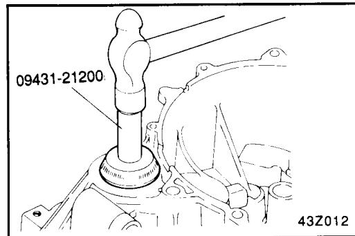
2. Install the input shaft front oil seal using the special tool (09431-21000).
