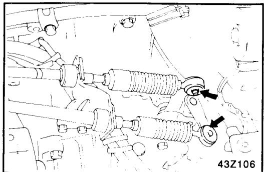
5. Separate the backup light switch connector.
