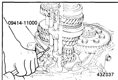
19. Disassembly of shift rail assembly.
