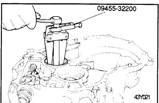
24. Remove the output shaft bearing outer race and spacer using the special tool (09455-32200).
