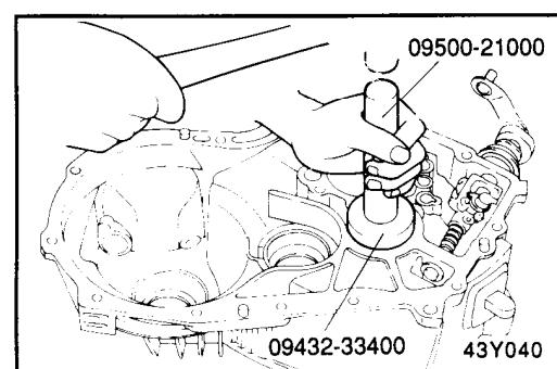
6. Install the differential gear assembly and output shaft assembly.
