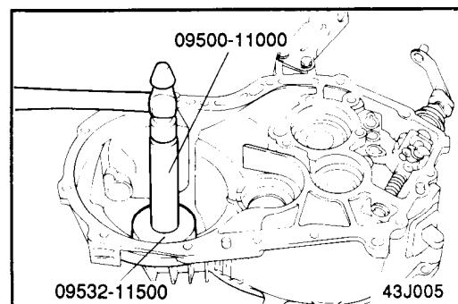
4. Install the output shaft bearing outer race and spacer using the special tool (09500-11000, 09532-11500).
