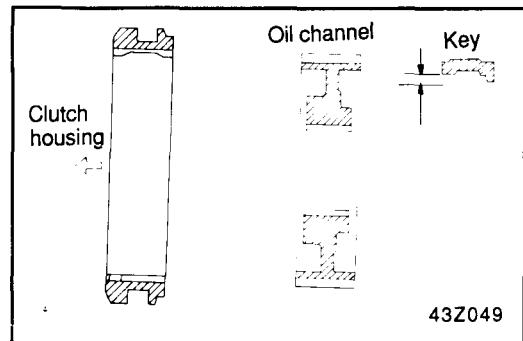
2. The synchronizer sleeve has teeth missing at six portions. Assemble the hub to the sleeve so that the center tooth between the two missing teeth will touch the synchronizer key.
