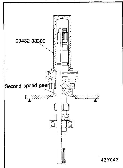
6. Install the needle roller bearing sleeve using the special tool (09432-33300).
