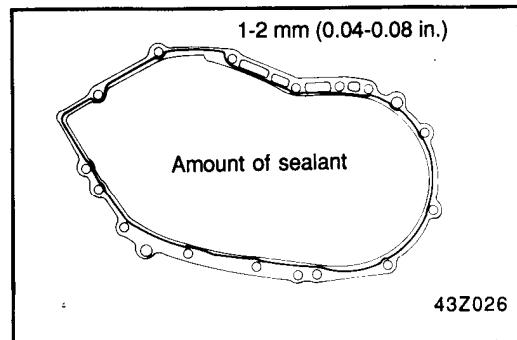
21. Install the transaxle case to the clutch housing assembly and tighten the (13) bolts.
