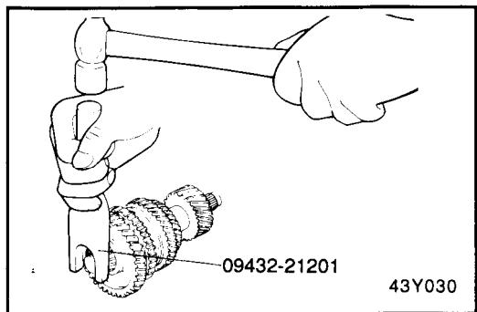
2. Remove the taper roller bearing, first speed gear and bearing sleeve and needle roller bearing using the special tool (09432-33100).
