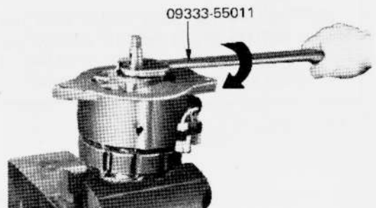
Fig. 7-48 Removing Bearing Lock Nut
