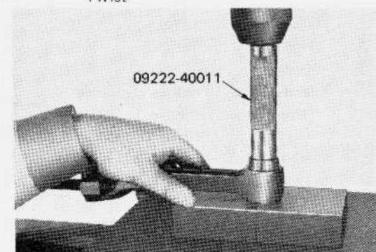
Fig. 2-69 Replacing Connecting Rod Bushing
