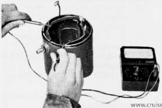
Fig. 7-17 Testing Field Coil for Ground
