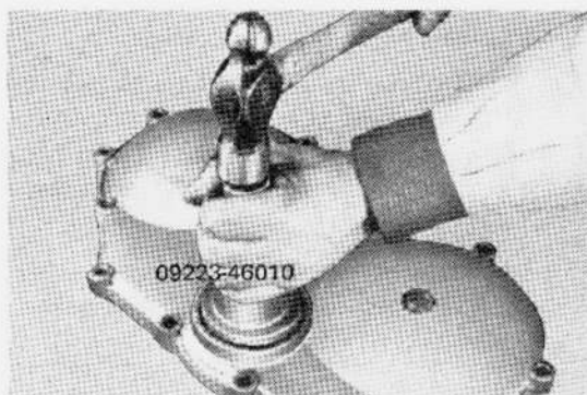
Fig. 2-86 Assembling Crankshaft Front Oil Seal
