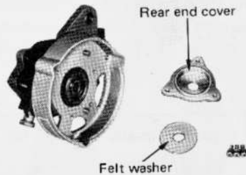
Fig. 7-76 Installing Felt Washer
