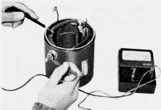
Fig. 7-16 Testing Field Coil for Open Circuit
