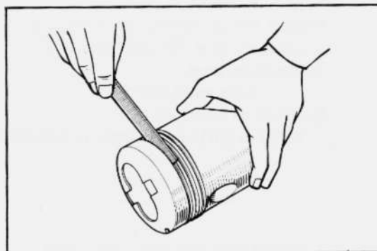
Fig. 2-65 Measuring Piston Ring to Groove Clearance
