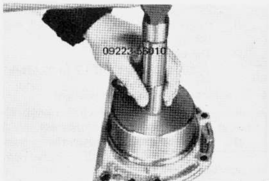
Fig. 2-87 Assembling Crankshaft Rear Oil Seal
