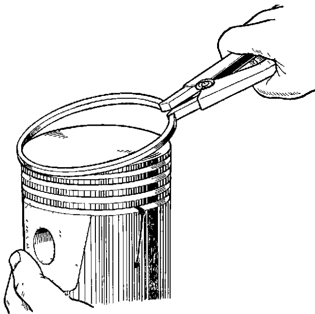
Figure 94 – Assembling Piston Rings to Piston
