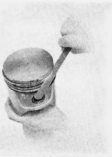
Figure 93 - Checking Piston Ring Clearance in Ring Groove
