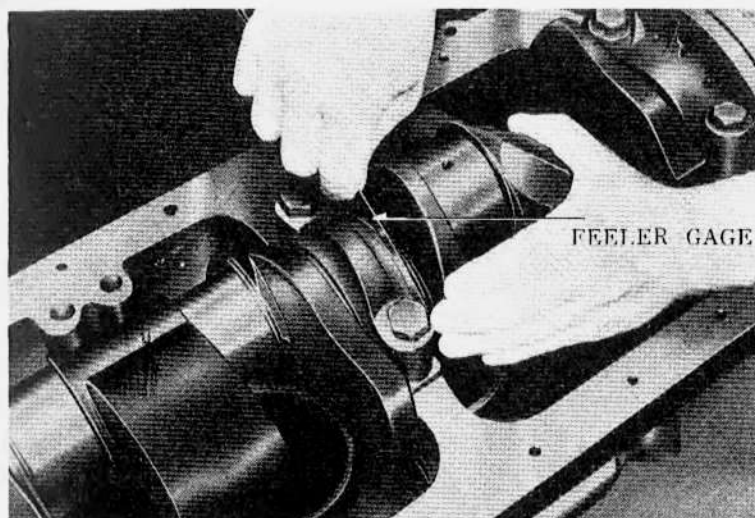
Figure 68—Checking Crankshaft End Play
