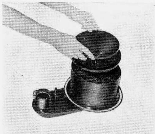
Figure 155 – Installing Wire Net and Baffle Plate
