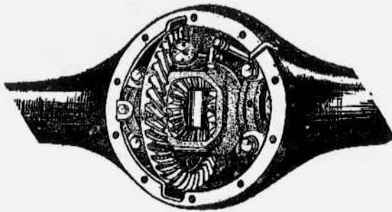
Measuring Backlash with Dial Gauge
