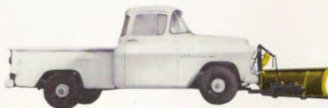
LST Light Duty Blade Snow Plow for 1/2-ton and pickup trucks.
