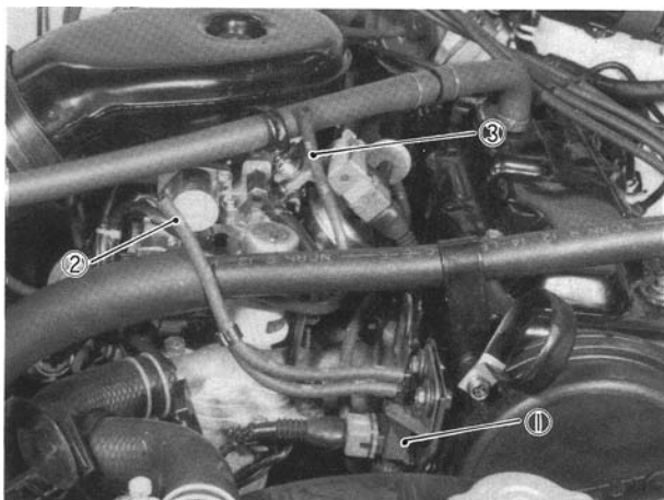
1. TWSV (Black) 3. To actuator 2. To intake manifold
