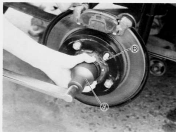
Fig. 17-5-23 Special Tool (A) (Front Wheel Bearing Nut Socket Wrench 09941-58010) Special Tool (B) (Automatic Free Wheeling Hub Socket 09944-98010)
