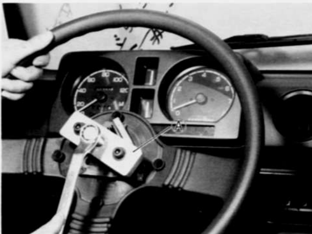
Fig. 7-6 (A) Special tool (Steering wheel remover 09944-38210)
