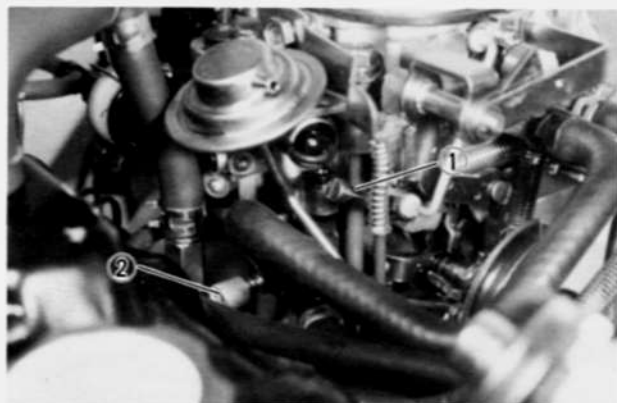
1. Idle speed adjusting screw 2. Idle mixture adjusting screw
