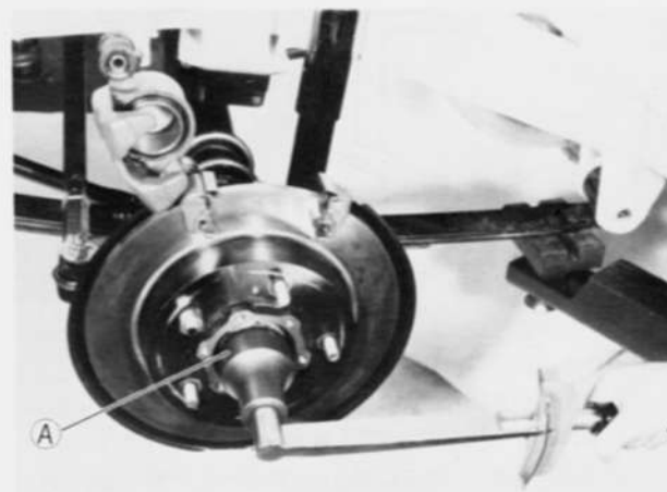
Fig. 17-3-8 (A) Special tool (Front Wheel Bearing nut socket wrench 09941-58010)
