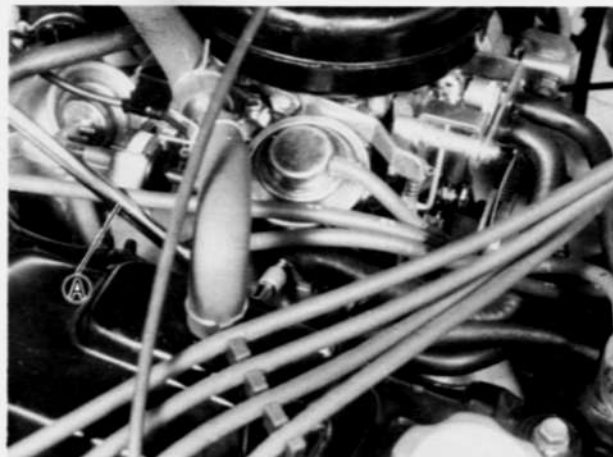
Fig. 4-1-35-1 ① Special Tool (Carburetor Adjuster 09918-38310)
