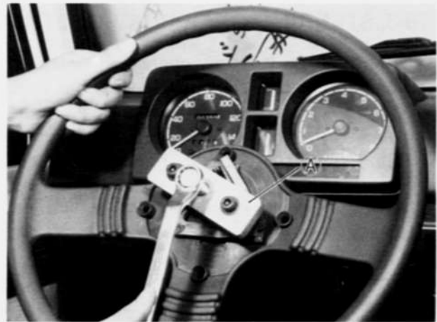
Fig. 18-4 Ⓐ Special tool (Steering wheel remover 09944-38210)
