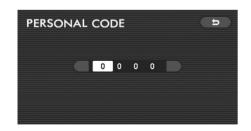
With an appropriate DVD video disc loaded in the player, access the SETUP MENU screen. Highlight "PARENTAL LOCK" with the remote control joystick, then press the "ENTER" button. The display will change to the "PERSONAL CODE" screen.
