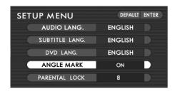
On the SETUP MENU screen, highlight "ANGLE MARK" with the remote control joystick, followed by pressing the "ENTER" button. Then, the angle mark display switches between "ON" and "OFF" each time the "ENTER" button is pressed. Select either "ON" or "OFF" as desired.
