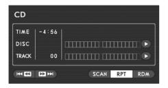
Highlight the "RTP" switch on the screen with the remote control joystick, then press the "ENTER" button.
