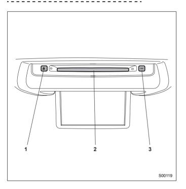
The DVD player can be operated when the ignition switch is in the "ACC" or "ON" position. Load a disc by inserting it into the disc slot of the player, with the label side facing up. The disc will be carried inward automatically when you insert it partially. The disc indicator light will turn on when the disc reaches the full inward position. To eject the disc, press the eject button. The disc will come out and the indicator light will go out.
