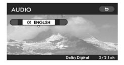
Click the "\(\nsigma\)" end of the remote control joystick to highlight the desired language on the screen and then press the "ENTER" button. To revert to the original video screen, highlight the "\(\sigma\)" switch with the joystick, and then press the "ENTER" button.
