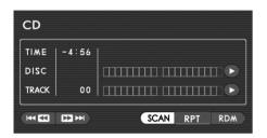
Highlight the "SCAN" switch on the screen with the remote control joystick, then press the "ENTER" button.
