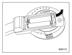
Remove the old batteries and install new ones (two AAA batteries). Pay careful attention to the (+) and (-) marks on the battery case.
