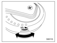
Adjust the sound level as desired with the volume dial on the right earpiece.
