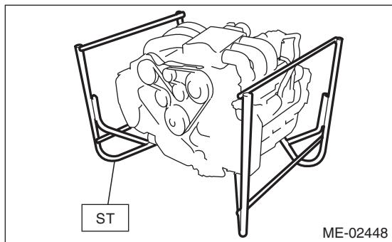
3) Before servicing overhaul, remove the sensor, pipe and hose that installed to engine.
