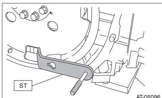
3) Tighten the drive plate mounting bolt.
