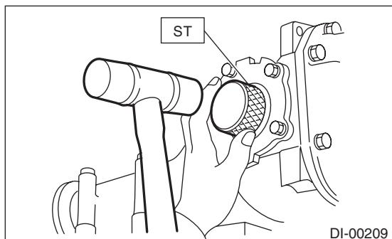
4) Install the rear differential. <Ref. to DI-20, INSTALLATION, Rear Differential (VA-type).>
