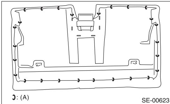
4) Remove the hog rings (A) on the front side of seat cushion.
