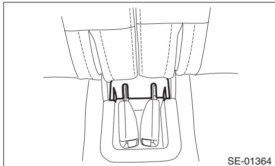
2) Lift up the front side of the 3rd seat cushion and then remove the hooks.
