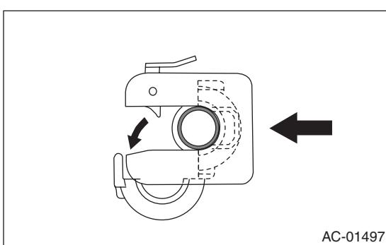
4. Pull the remover (2) and separate the pipe (3) from the quick connector (1).
