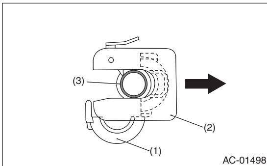
5. Pull up the stopper (C) and remove the remover (2) and quick connector (1) from the pipe.
