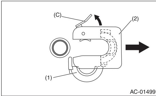
6. Disconnect the quick connector (1) from the remover (2).
