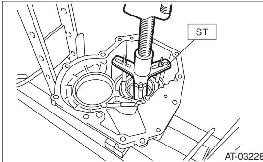
5) Install the transfer clutch. <Ref. to 5AT-65, INSTALLATION, Transfer Clutch.>
