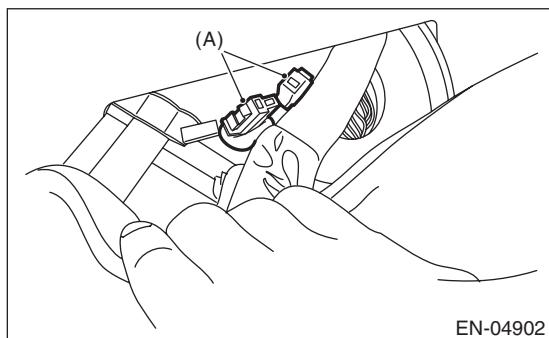
6) Connect SDI to data link connector located in the lower portion of the instrument panel (on the driver's side).
