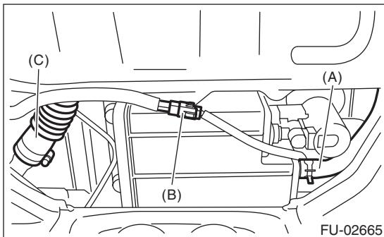
13) Remove the fuel tank from the vehicle.
