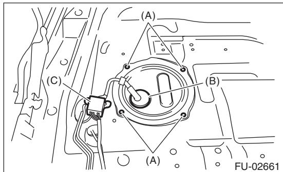
6) Remove the service hole cover of fuel sub level sensor.
