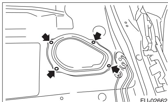
9) Install the service hole cover of fuel pump.
