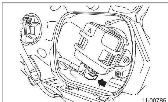
5) Remove the screws, and then remove the bulb.
