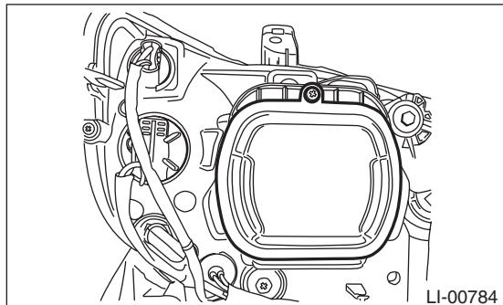
4) Remove the lock, and disconnect the harness connector.
