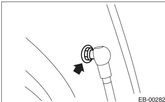
3) Remove mounting bolt, and remove the damper stay.
