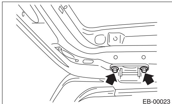
14) Remove the rear gate hinge from the vehicle.
