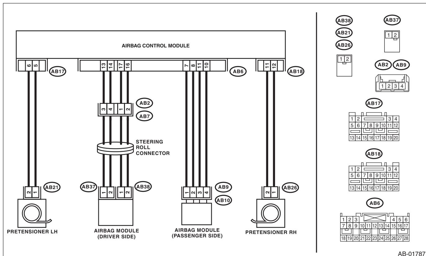
This DTC is indicated when the front airbag module and the pretensioner are deployed.
