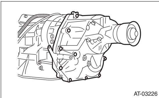
4) Remove the center differential carrier. <Ref. to 5AT-76, REMOVAL, Center Differential Carrier.>
