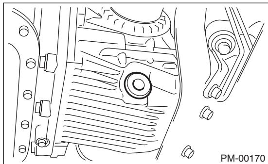
2) Replace the gasket with new part, and then tighten the drain plug to specified torque.
