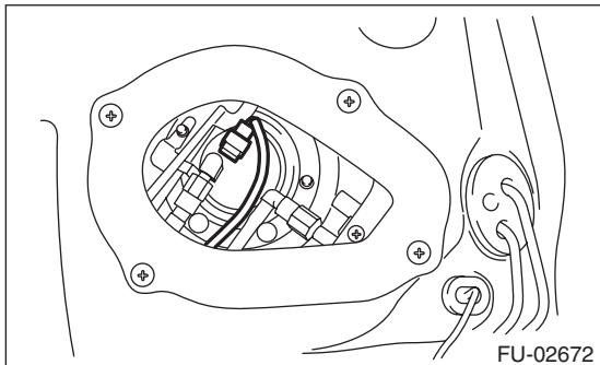
6) Disconnect the quick connector, and then disconnect the fuel delivery hose and jet pump hose. <Ref. to FU(H6DO)-54, REMOVAL, Fuel Delivery & Evaporation Lines.>
