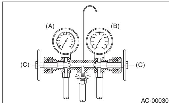
(A) Low-pressure gauge (Compound pressure gauge)
