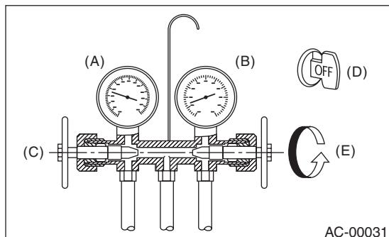
(A) Low-pressure gauge (Compound pressure gauge)
