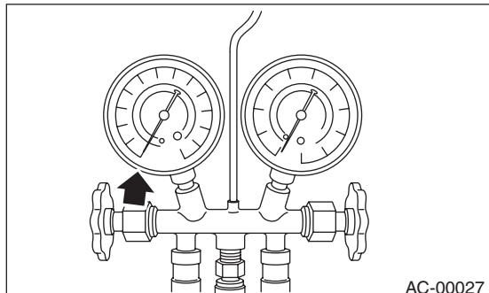
8) Leave it at least 5 minutes, and then check the low-pressure gauge reading for any changes.
