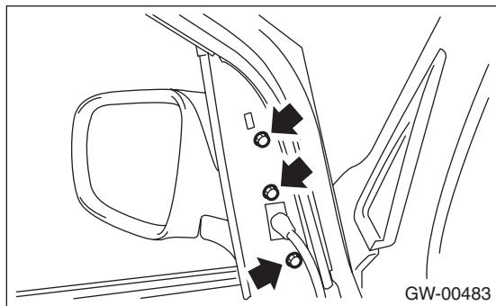
5) Remove the outer mirror assembly. (Model without door visor)
