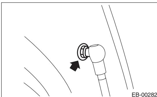
14) Remove the rear gate hinge bolt, and remove the rear gate panel.
