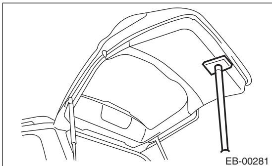
2) Remove the mounting bolt of rear gate damper stay.
