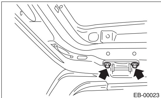
15) Remove the rear gate hinge from the vehicle.
