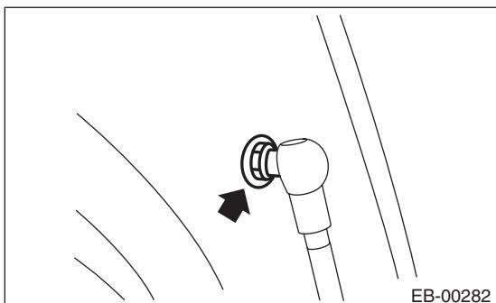
3) Remove the mounting bolts, and remove the damper stay.
