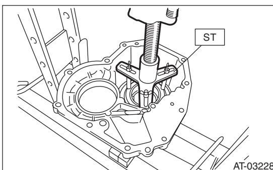
5) Install the transfer clutch. <Ref. to 5AT-67, INSTALLATION, Transfer Clutch.>
