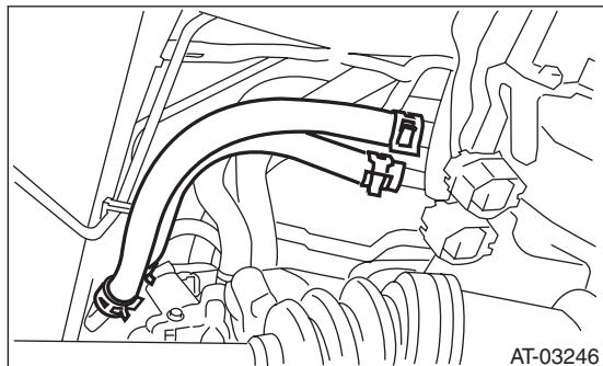
7) Connect the ATF cooler hose to the pipe on the radiator side.
