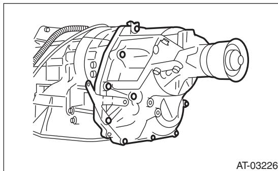
4) Remove the center differential carrier. <Ref. to 5AT-74, REMOVAL, Center Differential Carrier.>
