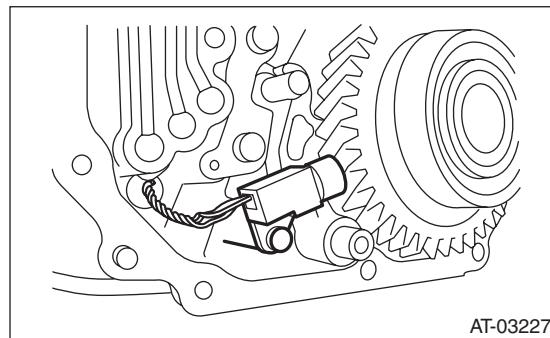
2) Connect the front vehicle speed sensor connector.
