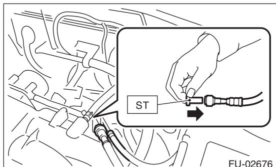
(2) Connect the fuel pressure meter using the ST2 and ST3.
