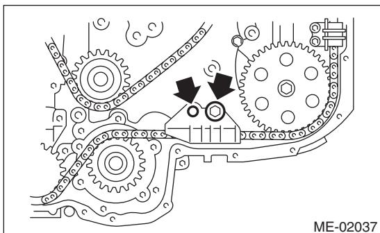
(6) Install the chain tensioner lever (LH).
