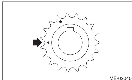
3) Align the key groove on exhaust cam sprocket to 12 o'clock position as shown in the figure.
