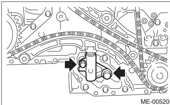
(7) Adjust the clearance between chain guide (RH) and chain guide (center) within 8.4 — 8.6 mm (0.331 — 0.339 in). Install the chain guide (center).
