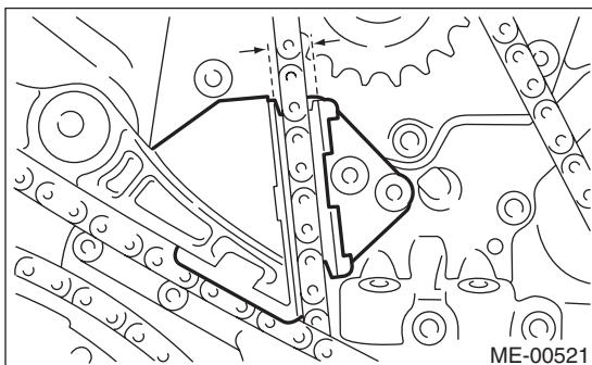
(8) Check that each mark on the sprocket and timing chain is matched, and then draw out the stopper pin from chain tensioner.
