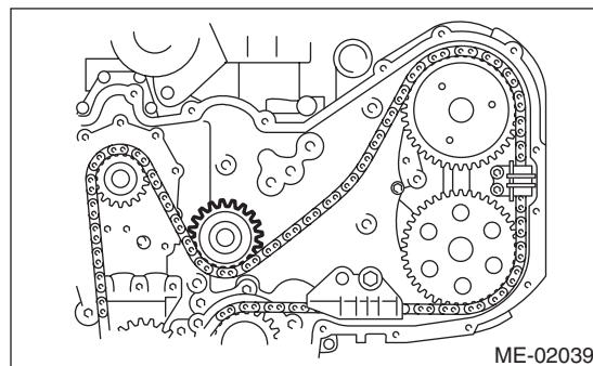
(4) Install the chain guide (LH: between cams).
