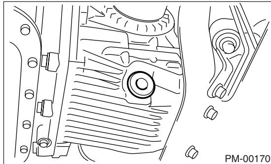
2) Replace the gasket with new one, and then tighten the drain plug to specified torque.
