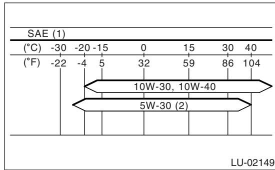
(1) SAE viscosity No. and applicable temperature
