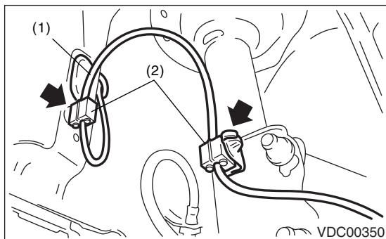
(1) To the front ABS wheel speed sensor connector
