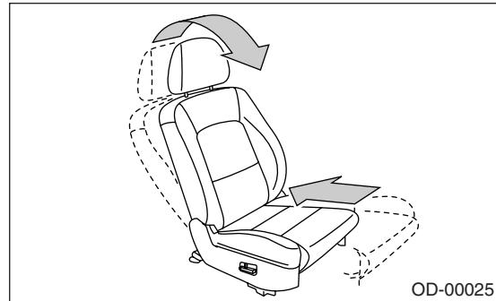
7) When the «Re-zeroing Unbelt the Passenger seatbelt Continue: YES, Quit: NO» is displayed, make sure the passenger's seatbelt is disconnected from the buckle and press the [YES] key.
