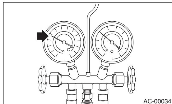
24) Adjust the refrigerant flow to maintain the pressure on the low-pressure side at 276 kPa (2.81 kg/cm<sup>2</sup>, 40 psi) max.
