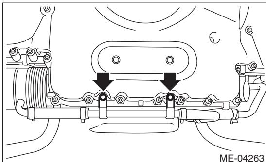
6) Install front mounting bracket to the cradle.
