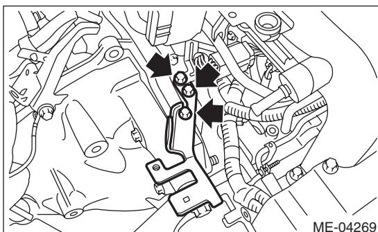
17) Install the engine harness connector to the engine hanger bracket.
