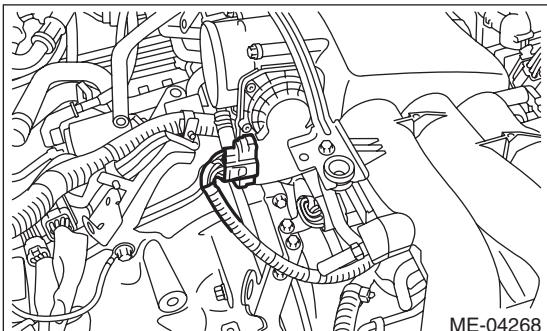
19) Connect the engine harness connector.
