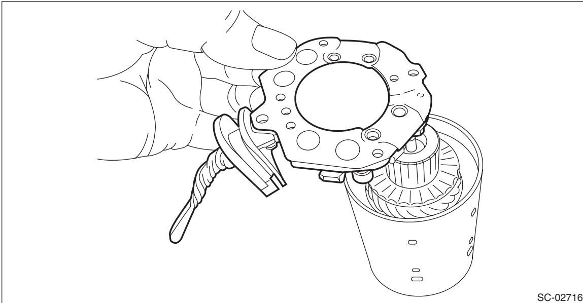
11) Remove the armature from the yoke.
