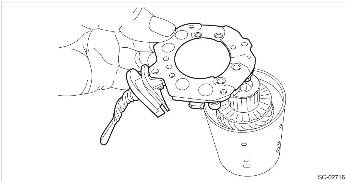
3) Install the starter cover, and secure it to the brush holder assembly with the screws.
