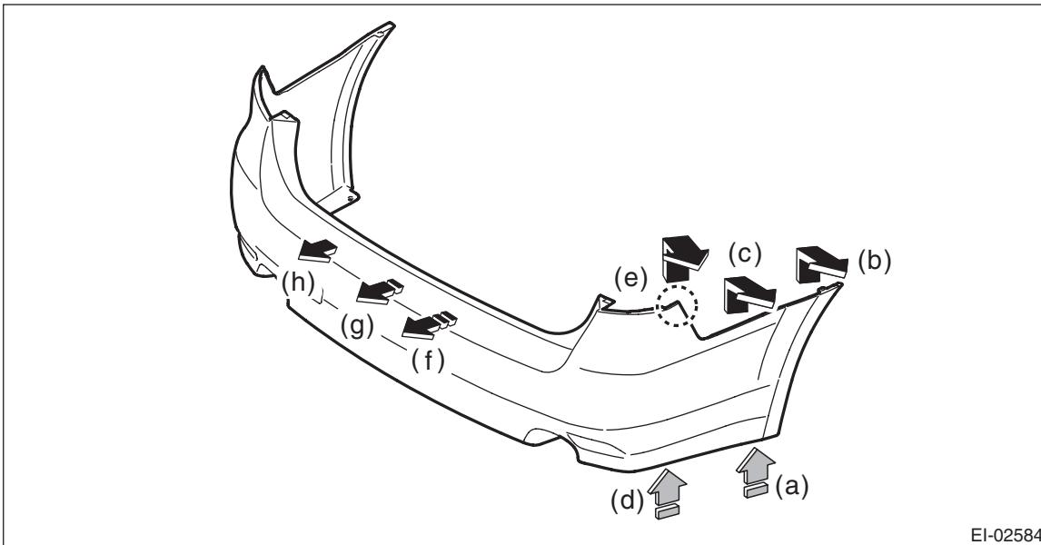
3) Remove the rear bumper beam assembly.
