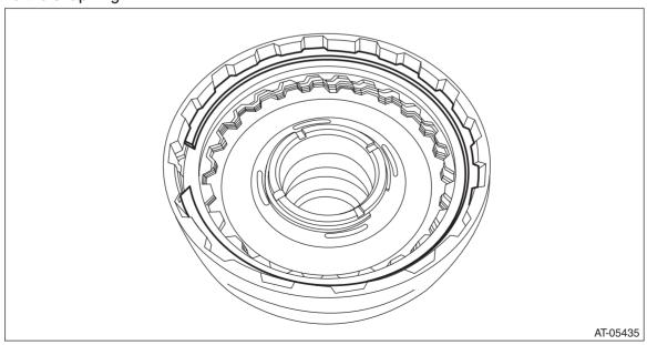
3) Remove the retaining plate, drive plate, driven plate and dish plate.
