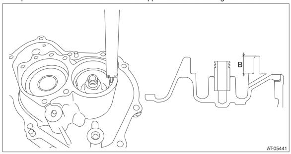
3) Measure depth "C" from the ST upper face to the bearing end face using the ST. ST 398643600 GAUGE
