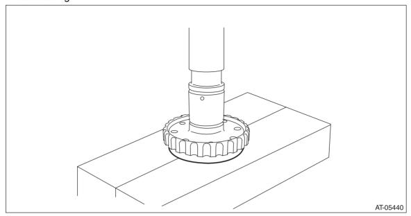
11) Install the seal ring to the front driven shaft.
