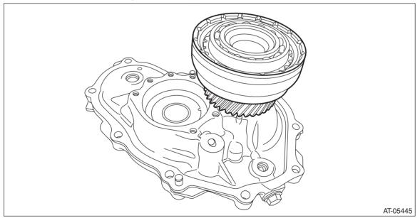
15) Apply compressed air intermittently to check the piston operation.
