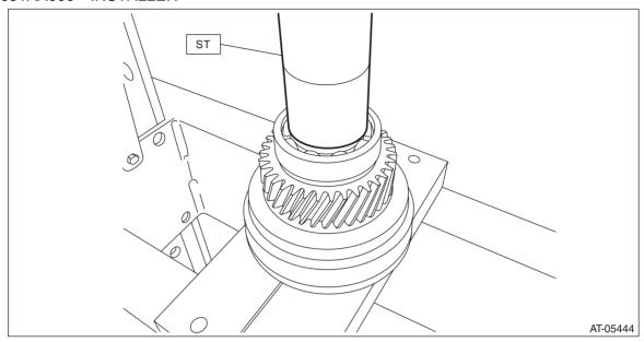
14) Install the front reduction driven gear assembly to converter case cover.
