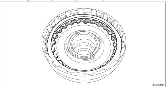
4) Remove the seal ring from front reduction driven shaft.
