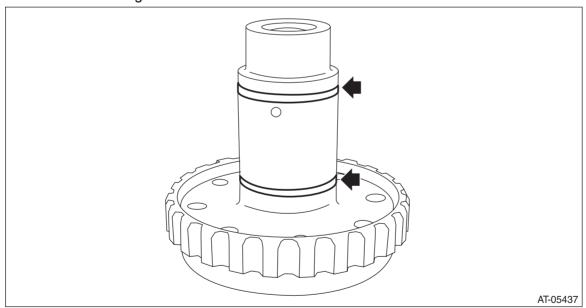
12) Install the front driven shaft to front driven gear.
