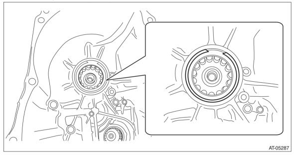
7) Using the ST, remove the roller bearing on primary pulley side.
