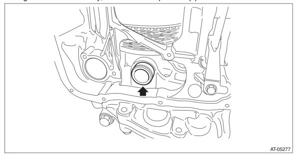
14) Remove the CVTF pipe using a tire lever etc.
