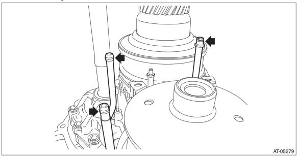
4) Make sure the lubrication pipe and support rod are in vertical position.
