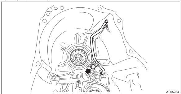
9) Install the CVTF inlet pipe and CVTF outlet pipe.
