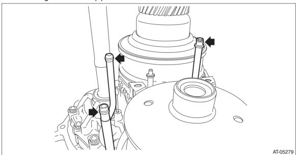
17) Remove the control device system. <Ref. to CVT-206, REMOVAL, Transmission Control Device.>
