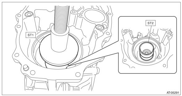
3) Using ST1 and ST2, install the roller bearing on primary pulley side.
