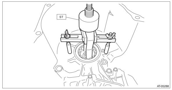
8) Remove the snap ring on secondary pulley side.
