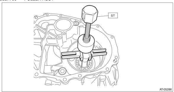
6) Remove the snap ring on primary pulley side.
