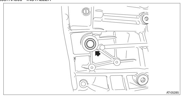
2) Using ST1 and ST2, install the ball bearing on the reduction gear side.
