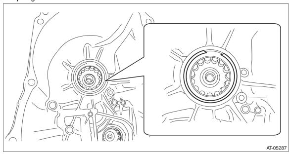
5) Using ST1 and ST2, install the roller bearing on secondary pulley side.
