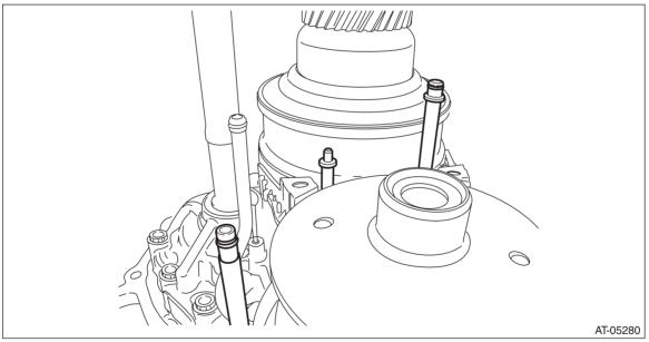
5) Apply liquid gasket seamlessly to the mating surface of transmission case.
