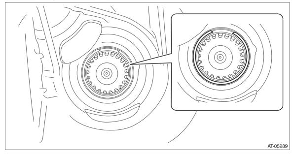
9) Using the ST, remove the roller bearing on secondary pulley side.
