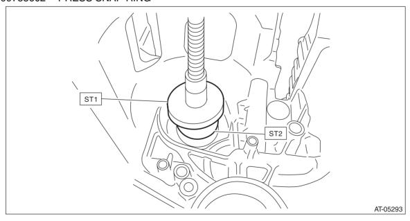
6) Install the snap ring on secondary pulley side.
