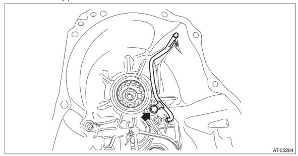
4) Remove the oil seal using a screwdriver wrapped with cloth etc.
