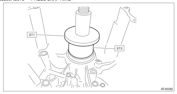
4) Install the snap ring on primary pulley side.
