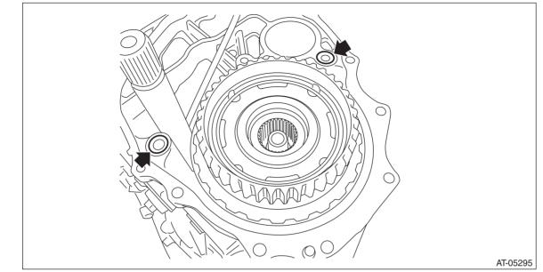
4) Apply liquid gasket to intermediate case seamlessly.
