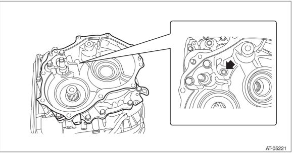
6) Install the transfer reduction driven gear assembly. <Ref. to CVT-157, INSTALLATION, Transfer Reduction Driven Gear.>
