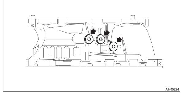
3) Remove the reverse brake assembly. <Ref. to CVT-170, DISASSEMBLY, Reverse Brake Assembly.>
