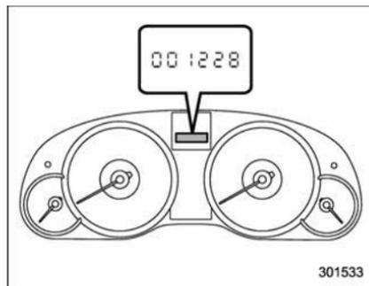
This meter displays the odometer when the ignition switch is in the "ON" position.
