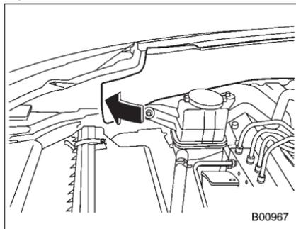
4. After replacing the bulbs, reposition the protective cover of the engine com-
