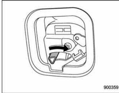
3. To unlock the rear gate, turn the lever to the right position using a flat-head screwdriver or a similar tool.
