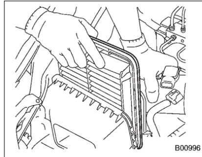
6. Open the air cleaner case and remove the air cleaner element.
