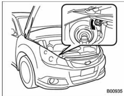
1. Turn the socket counterclockwise and pull it out.
