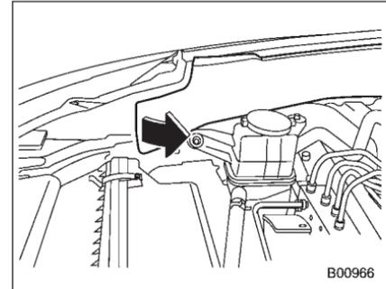
1. Turn over the protective cover of the engine compartment.
