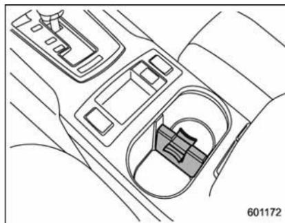
If you remove the divider plate from the dual cup holders, you can use the center console box as a storage space.
