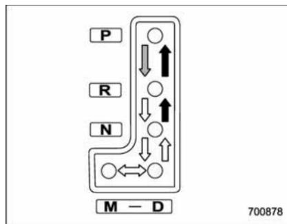
➡ : With the brake pedal depressed, shift while pressing the button in
