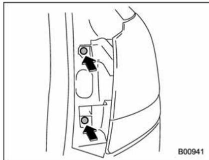
3. Remove the upper and lower screws.
