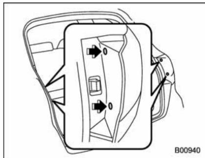
1. Undo the clips. For the method to undo the clips, refer to "Type C clips" Ⓞ 11-6.
