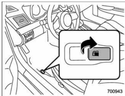
1. To open the fuel filler lid, pull the lid release lever up. The lever is on the floor at the left of the driver's seat.
