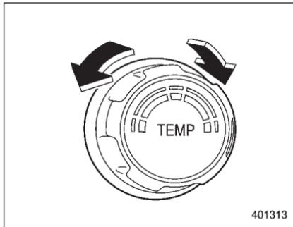
This dial regulates the temperature of airflow from the air outlets over a range from the blue side (cool) to red side (warm).
