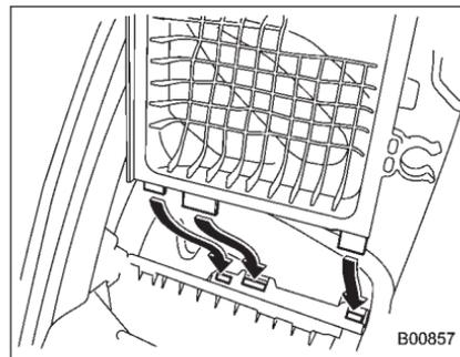
6. If the air cleaner case has been removed, insert the three projections on the air cleaner case into the slits on the air cleaner case cover.
