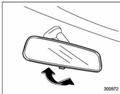
The mirror has a day and night position. Pull the tab at the bottom of the mirror toward you for the night position. Push it away for the day position. The night position reduces glare from headlights.
