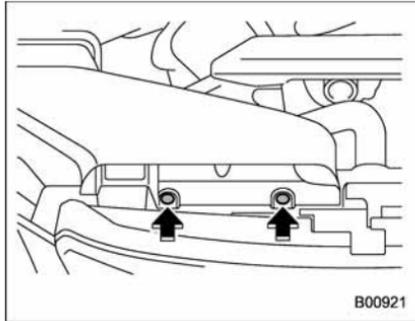
Use a screwdriver to undo the clips on the air intake duct, then remove the air intake duct. Refer to "Type A clips" ¶ 11-5.
