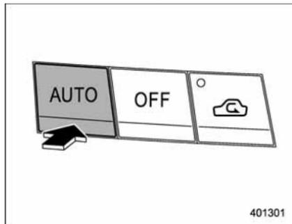
When the "AUTO" button is pressed, the indicator light "FULL AUTO" on the display illuminates. In this state, fan speed, airflow distribution, air-inlet control, and air conditioner compressor operation are automatically controlled.
