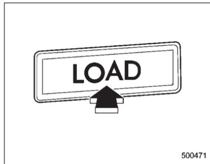
1. If you continue to press the "LOAD" button for more than 1.5 seconds, the player will produce beep sound and will enter the full disc loading mode.
