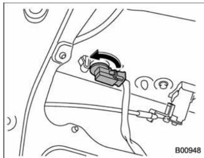
3. Turn the bulb socket counterclockwise and remove it.
