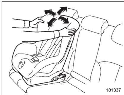
4. Before seating a child in the child restraint system, try to move it back and forth and left and right to verify that it is firmly secured in the center of the seat.
