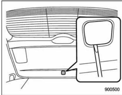
1. Remove the access cover at the bottom-center of the rear gate trim using flat-head screwdriver.
