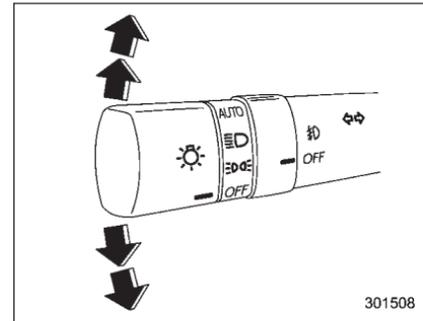
To activate the right turn signal, push the turn signal lever up. To activate the left turn signal, push the turn signal lever down. When the turn is finished, the lever will return automatically. If the lever does not return after cornering, return the lever to the neutral position by hand.
