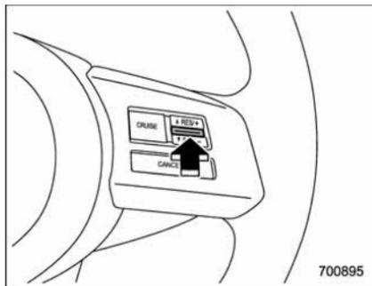
To resume the cruise control after it has been temporarily canceled and with vehicle speed of approximately 20 mph (32 km/h) or more, press the "RES/SET" switch to the "RES" side to return to the original cruising speed automatically.
