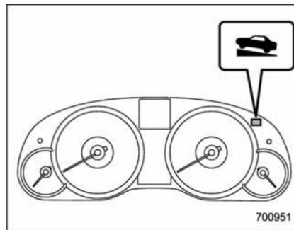
When the Hill Holder function is activated, the Hill Holder indicator light illuminates. Refer to "Hill Holder indicator light" 3-19.
