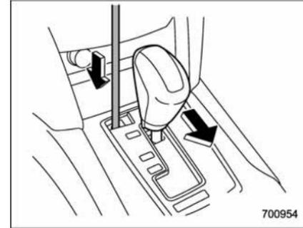
3. While depressing the brake pedal, insert the electronic parking brake release tool into the hole, press the shift lock release button using the tool, and then move the select lever.
