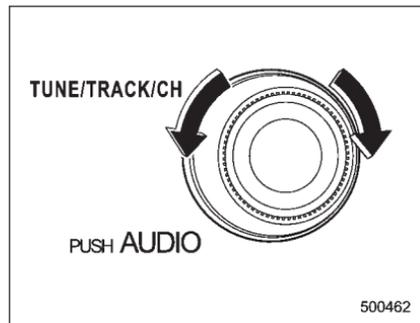
Turn the "TUNE/TRACK/CH" dial clockwise to select the next channel and turn the "TUNE/TRACK/CH" dial counterclockwise to select the previous channel.
