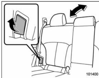
Pull the lever and adjust the seatback to the desired position.
