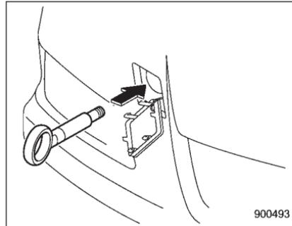
3. Screw the towing hook into the threaded hole until the threads can no
