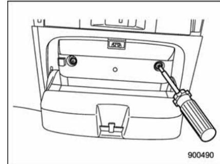
3. Remove the two screws that retain the moonroof switch body. Then, remove the moonroof switch.
