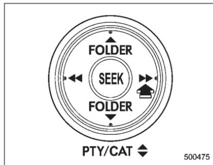
Press the “▶▶” side of the “SEEK” button continuously to fast-forward the track/file. Release the button to stop fast-forwarding.
