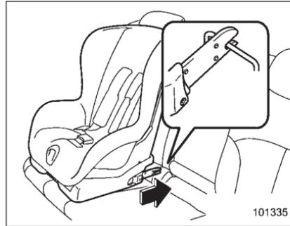
1. While following the instructions supplied by the child restraint system manufacturer, connect the lower hooks onto the lower anchorages located at "Ⓞ" marks on the bottom of the rear seatback. When the hooks are connected, make sure the adjacent seatbelts are not caught.
