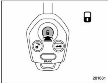
Press the “
