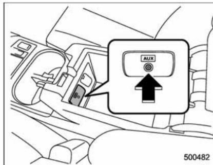
By connecting a commercial audio product to the vehicle, such as a portable audio player, you can hear its sound via the vehicle's speaker.
