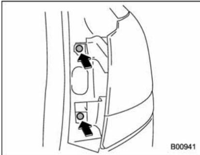
9. Tighten the upper and lower screws.
