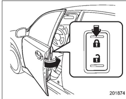
6. Press the front side (“LOCK” side) of the power door locking switch to set the door locks.
