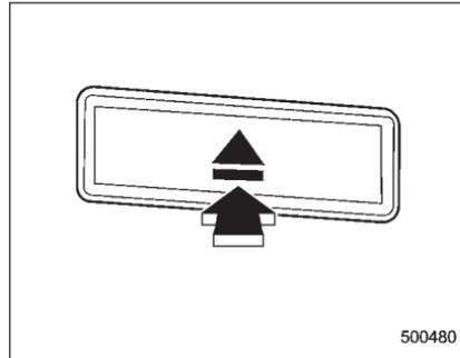
1. If you press the “▲” button for 1.5 seconds or longer, the player will produce beep sound and will enter the all disc ejection mode. At this time, the disc number indicator and “ALL EJECT” indicator will flash.
