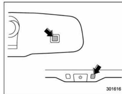
The mirror has a photosensor attached on the front and back sides. During nighttime driving, these sensors detect distracting
