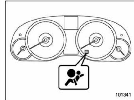
A diagnostic system continually monitors the readiness of the SRS airbag system (including front seatbelt pretensioners) while the vehicle is being driven. The SRS airbag system warning light will show normal system operation by illuminating for approximately 6 seconds when the ignition switch is turned to the "ON" position.
