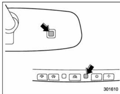
The mirror has a photosensor attached on both the front and back sides. During nighttime driving, these sensors detect distracting glare from vehicle headlights behind you and automatically dim the mirror to eliminate glare and preserve your vision. For this reason, use care not to cover the sensors with stickers, or other similar items. Periodically wipe the sensors clean using a piece of dry soft cotton cloth or an applicator.
