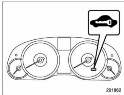
The security indicator light deters potential thieves by indicating that the vehicle is equipped with an immobilizer system. It begins flashing approximately 60 seconds after the ignition switch is turned from the "ON" position to the "Acc" or "LOCK" position or immediately after the key is pulled out.
