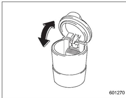
The portable ashtray can be installed in each cup holder. For the locations of the cup holders, refer to "Cup holder" 6-8. When using the ashtray, open the lid of the ashtray. When removing the ashtray from a cup holder, pull the ashtray upwards.
