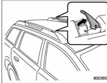
1. Pull out the integrated crossbars from the roof rail holders by pulling up the covers.
