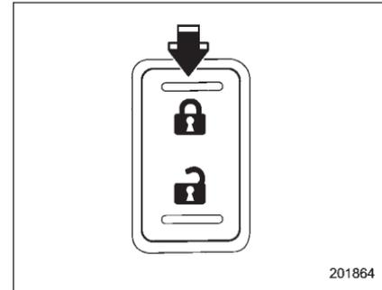
5. Before the electronic tone stops sounding, press the lock side of the power door lock switch the same number of times as the leftmost digit of the transmitter code. For example, press the lock switch eight times if the leftmost digit of the code is 8.
