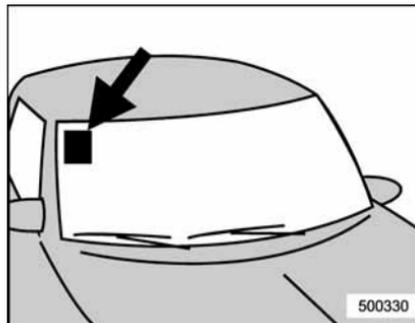
For some models, the satellite radio antenna is fixed to the upper right hand corner of the windshield.
