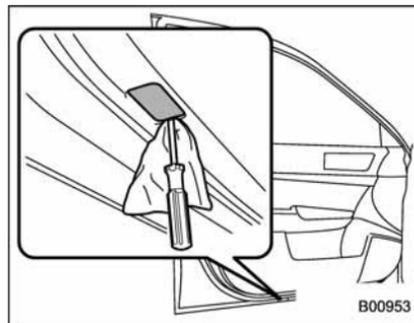
1. Remove the lens by prying the edge of the lens with a flat-head screwdriver.
