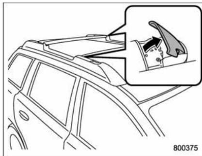
1. Pull out the crossbars from the roof rail holders by pulling up the covers.
