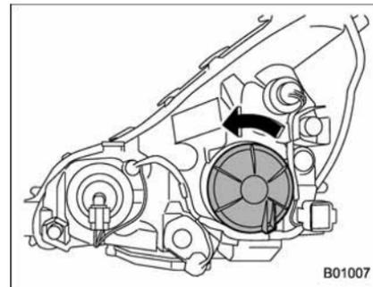
2. Remove the bulb cover, by turning it
