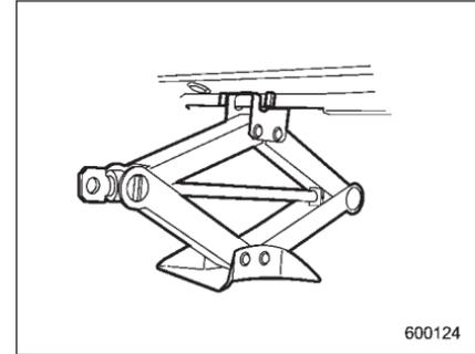
Turn the jackscrew by hand until the jack head engages firmly into the jack-up point.
