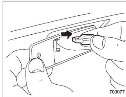
3. Pull the bulb out of the socket.
