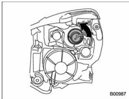
2. Turn the socket counterclockwise and pull it out.
