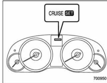
At this time, the cruise control set indicator light is illuminated in the combination meter.
