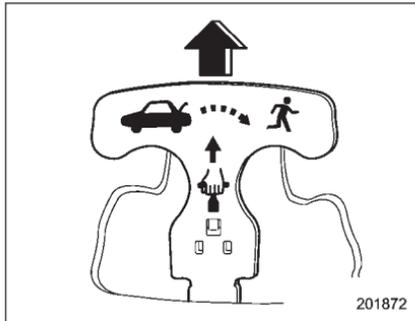
To open the trunk lid from inside the trunk, pull the yellow handle as indicated by the arrow on the handle. This operation unlocks the trunk lid. Then, push up the lid.
