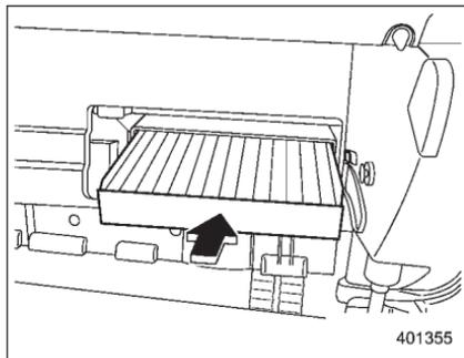
4. Replace the air filter element with a new one.
