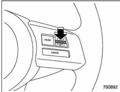
3. Press the "RES/SET" switch to the "SET" side and release it. Then release
