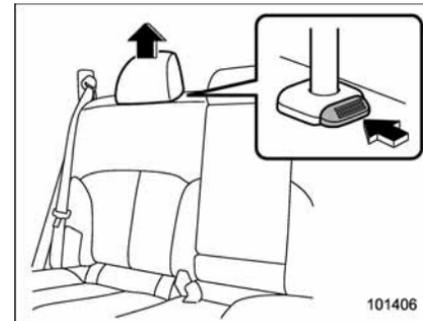
1. Remove the head restraint at the seating position where the child restraint system has been installed with the seatbelt or lower anchorages; lift up the head restraint while pressing the release button. Store the head restraint in the cargo area. Avoid placing the head restraint in the passenger compartment to prevent it from being thrown around in the passenger compartment in a sudden stop or a sharp turn.
