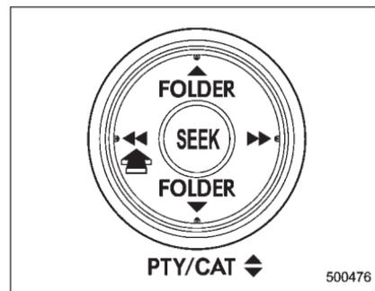
Press the “◀◀” side of the “SEEK” button continuously to fast-reverse the track/file. Release the button to stop fast-reversing.
