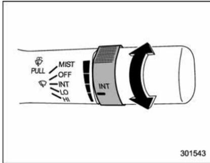
When the wiper switch is in the “INT” position, turn the dial to adjust the operating interval of the wiper. The operating interval can be adjusted in five steps from the shortest interval to the longest.
