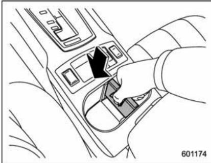
Insert the divider plate into the console box.
