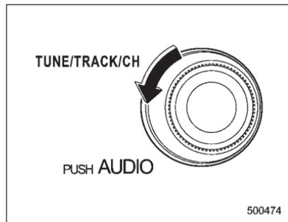
Turn the “TUNE/TRACK/CH” dial counter-clockwise to skip to the beginning of the current track/file (track). Each time the dial is turned, the indicated track/file (track) number will decrease.
