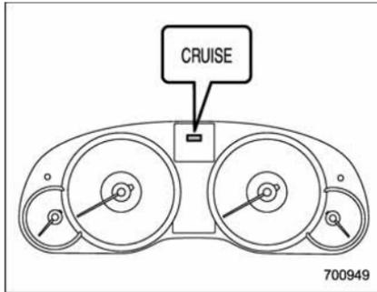
The cruise control indicator light on the combination meter will illuminate.
