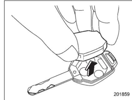
3. Remove the transmitter case from the key head.
