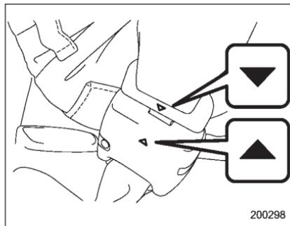
4. After fastening the seatbelt, make sure that the “▼” mark on the connector (tongue) and the “▲” mark on the buckle face outwards.
