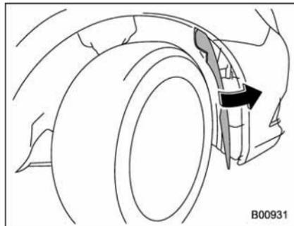
8. After replacing the bulb, reattach the fender lining.
