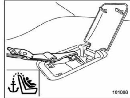
4. Fasten the top tether hook of the child restraint system to the appropriate upper anchorage.
