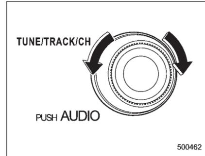
Turn the “TUNE/TRACK/CH” dial clockwise to increase the tuning frequency and turn the “TUNE/TRACK/CH” dial counter-clockwise to decrease it.
