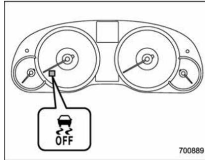
The light illuminates when the ignition switch is turned to the "ON" position and turns off after approximately 2 seconds. The light illuminates when the Vehicle Dynamics Control OFF switch is pressed to deactivate the Vehicle Dynamics Control system.
