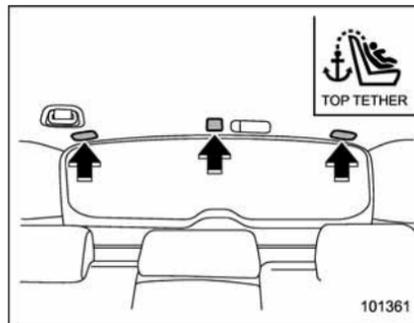
Three tether anchorages, i.e., ones for the right, center and left positions, are already installed on the rear edge of the roof. Open the cover flap to use each anchorage.
