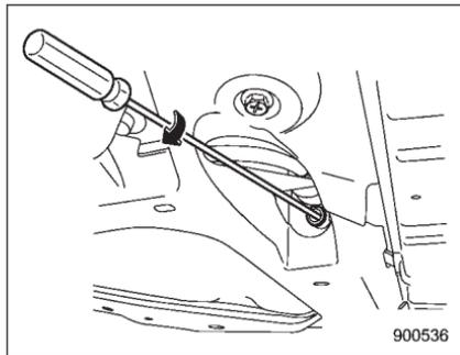
8. Break the white film and insert the electronic parking brake release tool into the parking brake release device.
