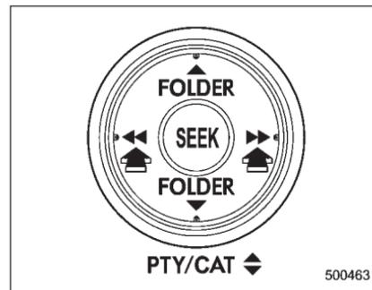
When in the SAT mode, press the "SEEK" button "◀◀" or "▶▶" continuously to change to the channel selection mode. Pressing the "SEEK" button "▶▶" changes the channel up by 10 steps each time. Pressing "◀◀" changes the channel down by 10 steps each time.
