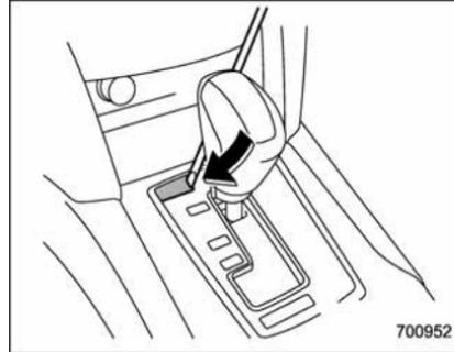
2. Remove the shift lock cover using a flat-head screwdriver.
