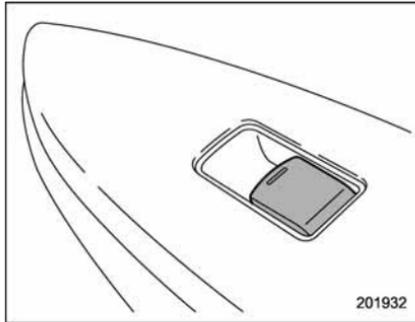
Each passenger window can be controlled by the power window switch located on the door.
