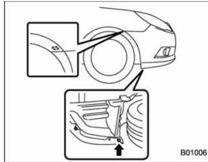
3. Remove the clip from the fender lining. Refer to "Type B clips" ¶ 11-5.
