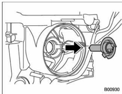
5. Replace the bulb, then set the retainer spring securely.
