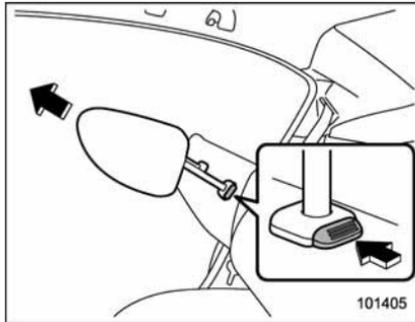
2. Remove the head restraint at the seating position where the child restraint system has been installed with the seatbelt or lower anchorages; lift up the head
