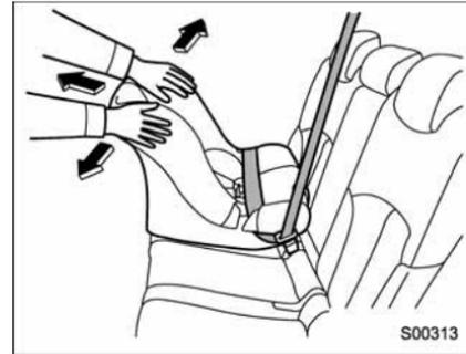
6. Push and pull the child restraint system forward and side to side to check that it is firmly secured in the center of the seat.
