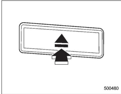
2. Briefly press the “▲” button. The selected disc will be ejected. The disc number indicator will flash at this time. When you remove the ejected disc, the disc number indicator will turn off.
