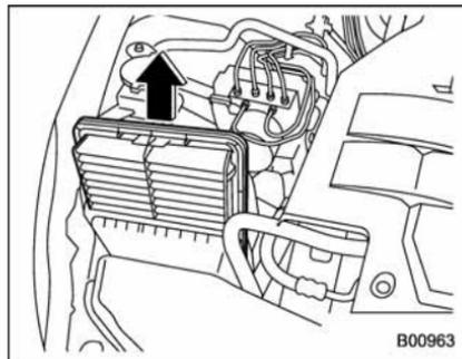
4. Open the air cleaner case and remove the air cleaner element.
