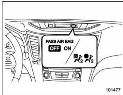
ON or Front passenger's frontal airbag ON indicator
