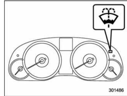
The windshield washer fluid warning light illuminates when the washer fluid level in the tank has dropped to the lower limit. If the warning light illuminates, refill the tank with fluid. For the tank refilling method, refer to “Windshield washer fluid” 11-41.
