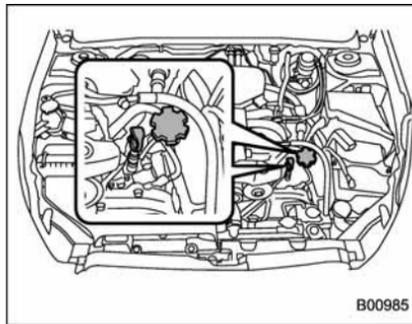
2. Pull out the level gauge, wipe it clean, and insert it again.
