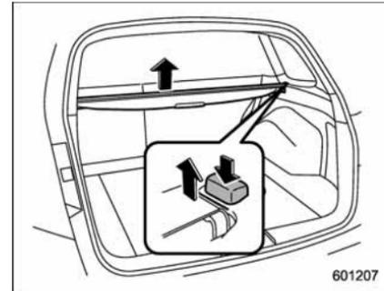
2. Hold down the button on the right-hand rear quarter panel and lift up the right-hand cover housing.
