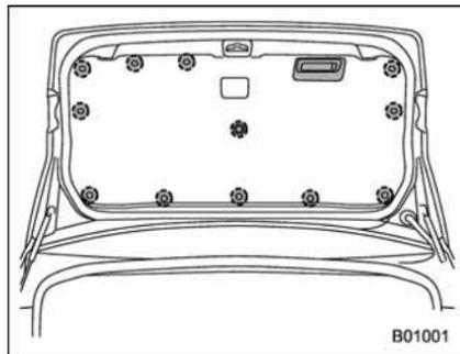
2. Remove the trunk trim lining by removing the 12 clips and the trunk trim handle.
