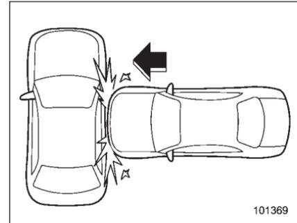
A severe side impact near the front seat or the rear seat activates the SRS curtain airbag.
