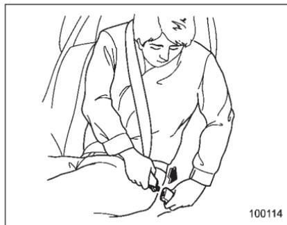
5. Insert the center seatbelt tongue plate into the center seatbelt buckle marked
