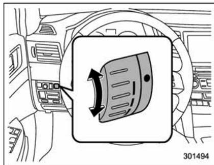
The illumination brightness of the clock display, audio, air conditioner, multi function display and meter/gauge dims under the following conditions.
