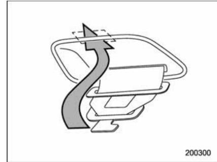
2. Allow the retractor to roll up the belt. You should hold the webbing end and guide it back into the retractor while it is rolling up. Neatly store the tongue plate in the recess and then insert the connector (tongue) plate into the slot.
