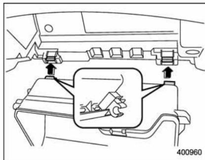
6. Reinstall the glove box, and connect the damper shaft.
