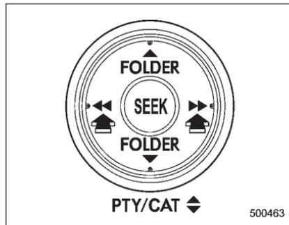
When in the SAT mode, briefly press the "SEEK" button "◀◀" or "▶▶" to select the channel.
