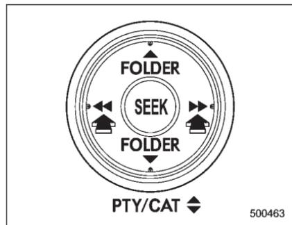
If you press the "◀◀" or "▶▶" side of the "SEEK" button briefly, the radio will automatically search for a receivable station and stop at the first one it finds. This function may not be available, however, when radio signals are weak. In such a situation, perform manual tuning to select the desired station.
