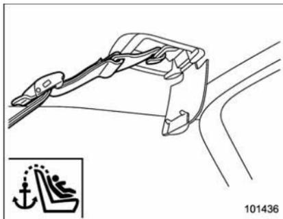
3. Fasten the top tether hook of the child restraint system to the appropriate upper anchorage.
