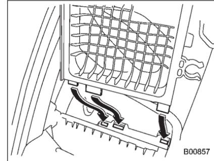
8. To install the air cleaner case, insert the three projections on the air cleaner case into the slits on the air cleaner case cover.
