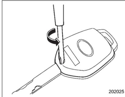
1. Remove the screw on the key head.
