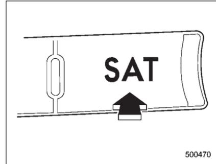
Press the "SAT" button when the radio is off to turn on the radio.
