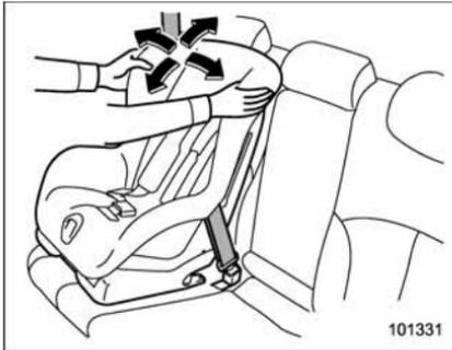
6. Before seating a child in the child restraint system, try to move it back and forth and left and right to verify that it is firmly secured in the center of the seat. Sometimes a child restraint can be more firmly secured by pushing it down into the seat cushion and then tightening the seatbelt.
