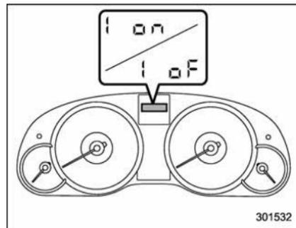
It is possible to activate or deactivate the movement of the meter needles and gauge needles that takes place when the ignition switch is turned to the "ON" position.
