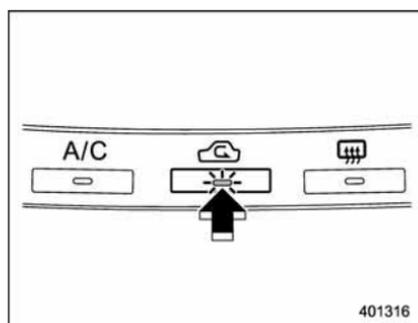
**ON position (recirculation):** Interior air is recirculated inside the vehicle.
