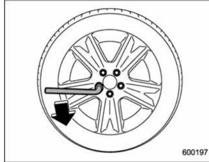
7. Loosen the wheel nuts using the wheel nut wrench but do not remove the nuts.
