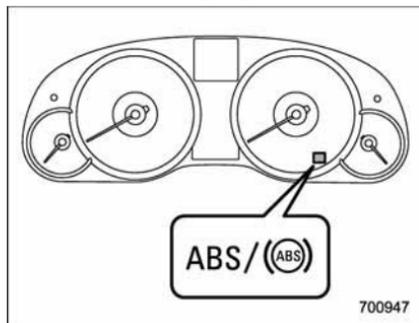
The ABS warning light illuminates when the ignition switch is turned to the "ON" position and turns off after approximately 2 seconds.
