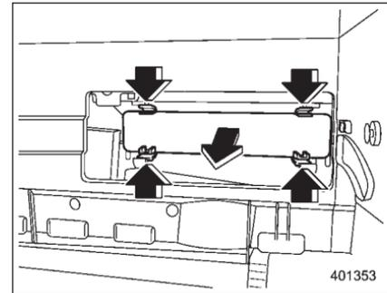
2. Remove the cover of the air filter.
