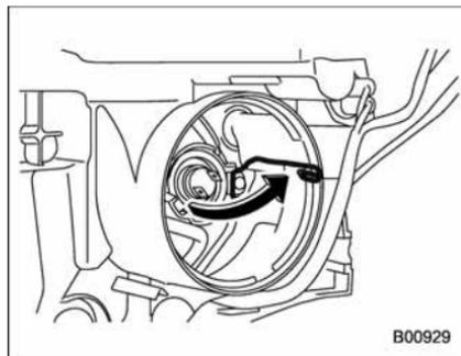
4. Remove the retainer spring.
