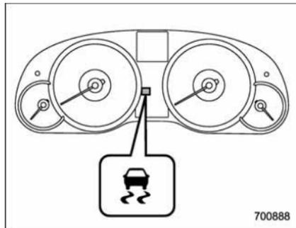
The light illuminates when the ignition switch is turned to the "ON" position and turns off several seconds after the engine has started. This lighting pattern indicates that the Vehicle Dynamics Control system is operating normally.
