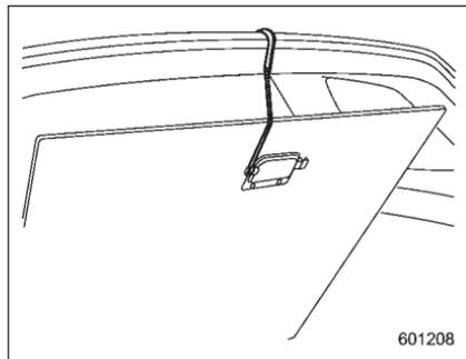
2. To keep the lid open, hang the hook (provided on the back of the lid) on the rear edge of the roof.
