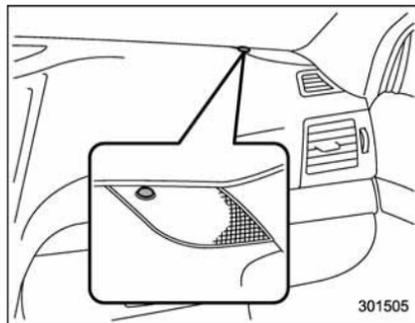
The sensor is on the instrument panel as shown in the illustration.
