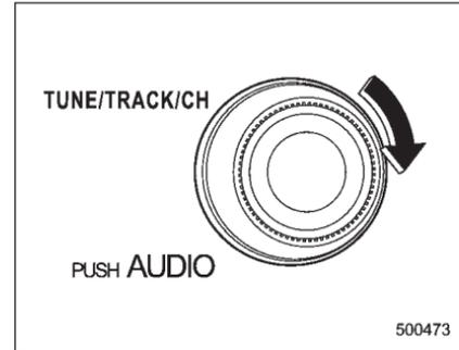
Turn the “TUNE/TRACK/CH” dial clockwise to skip to the beginning of the next track/file (track). Each time the dial is turned, the indicated track/file (track) number will increase.
