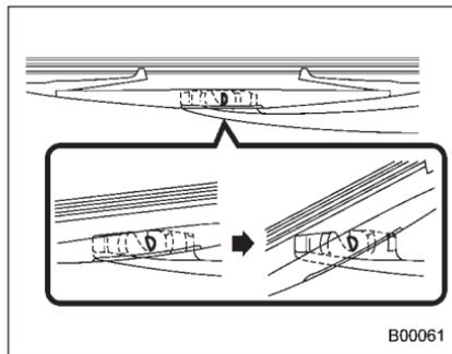
2. Turn the wiper blade assembly counterclockwise.
