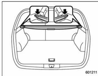
1. To install the cover housing, insert both ends of the cover housing into the retainers.
