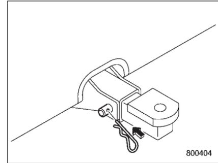
3. Insert the safety pin onto the hitch pin securely.
