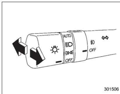
To change from low beam to high beam, push the turn signal lever forward. When the headlights are on high beam, the high beam indicator light "☰●" on the combination meter is also on.
