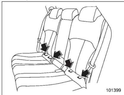
The lower anchorages (bars) are used for installing a child restraint system only on
