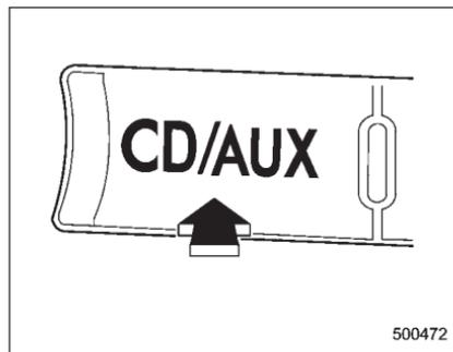
2. Press the AUX input selection button "CD/AUX" on the audio control panel to turn on the auxiliary audio input.
