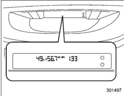
With the ignition switch in the "ON" position, each successive press of the multi function display switching knob toggles the display in the following sequence.
