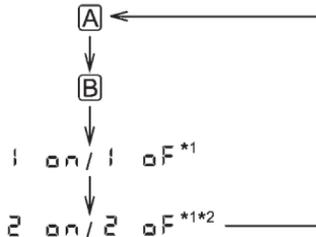
\*1: "1 ON" or "1 OFF" and "2 ON" or "2 OFF" cannot be displayed when the ignition switch is in the "ON" position.
