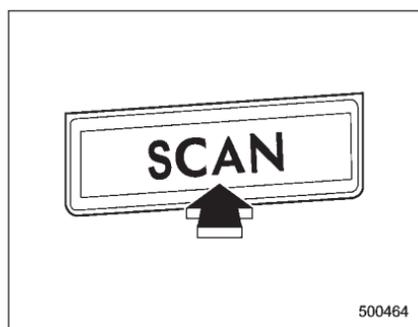
If you press the "SCAN" button, the radio will switch to the scan mode. In this mode, the radio scans through the radio band until a station is found. The radio will stop at the station for 5 seconds while displaying the frequency, after which scanning will continue until the entire band has been scanned.
