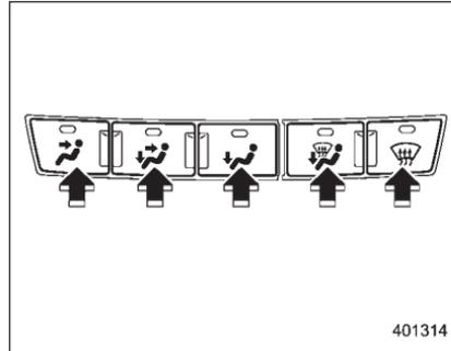
Each airflow control button activates the following air outlets.
