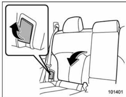
Unlock the seatback by pulling the release lever and then fold the seatback down.
