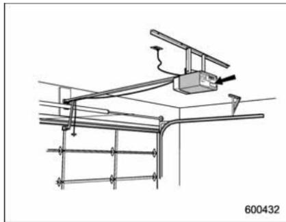
1. Locate the training button on the garage door opener motor head unit. The exact location and color of the button may vary by brand of garage door opener. If it is difficult to locate the training button, refer to your garage door opener’s instruc-
