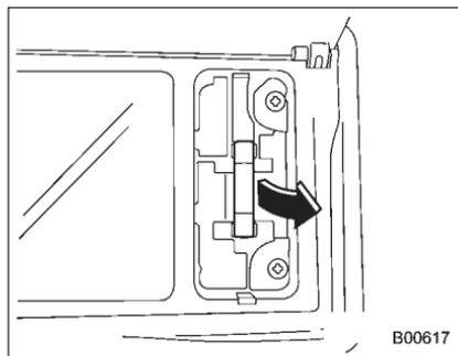
2. Pull the bulb out of the socket.
