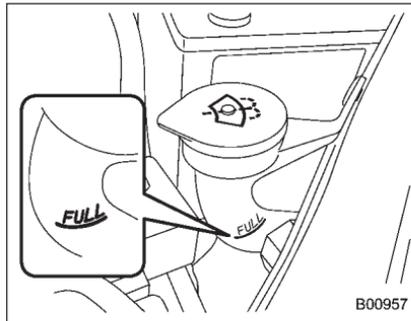
Remove the washer tank filler cap, then add fluid until it reaches the "FULL" mark on the tank.
