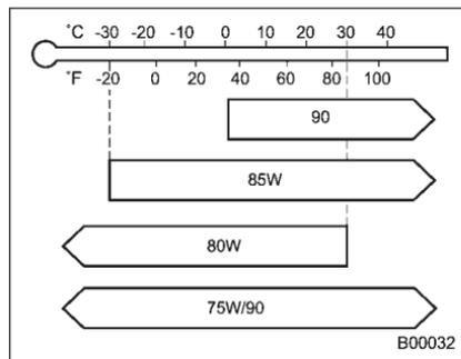
SAE viscosity No. and applicable temperature
