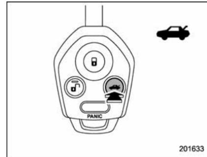
The trunk lid opens when the “
