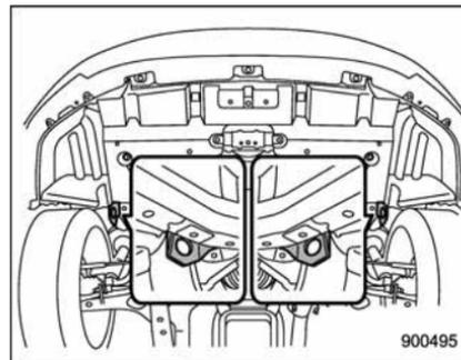
The front tie-down hooks are located between each of the front tires and the front bumper.
