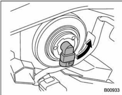
4. Remove the bulb from the headlight assembly by turning it counterclockwise.
