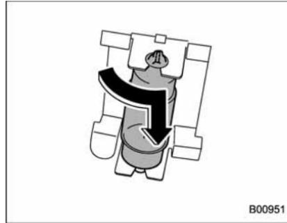
2. Turn the bulb until the flat surfaces at its ends are aligned vertically.
