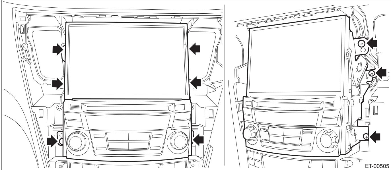
5) Remove the control panel assembly.
