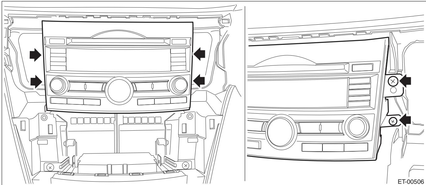
4) Remove the navigation assembly. (model with navigation)
