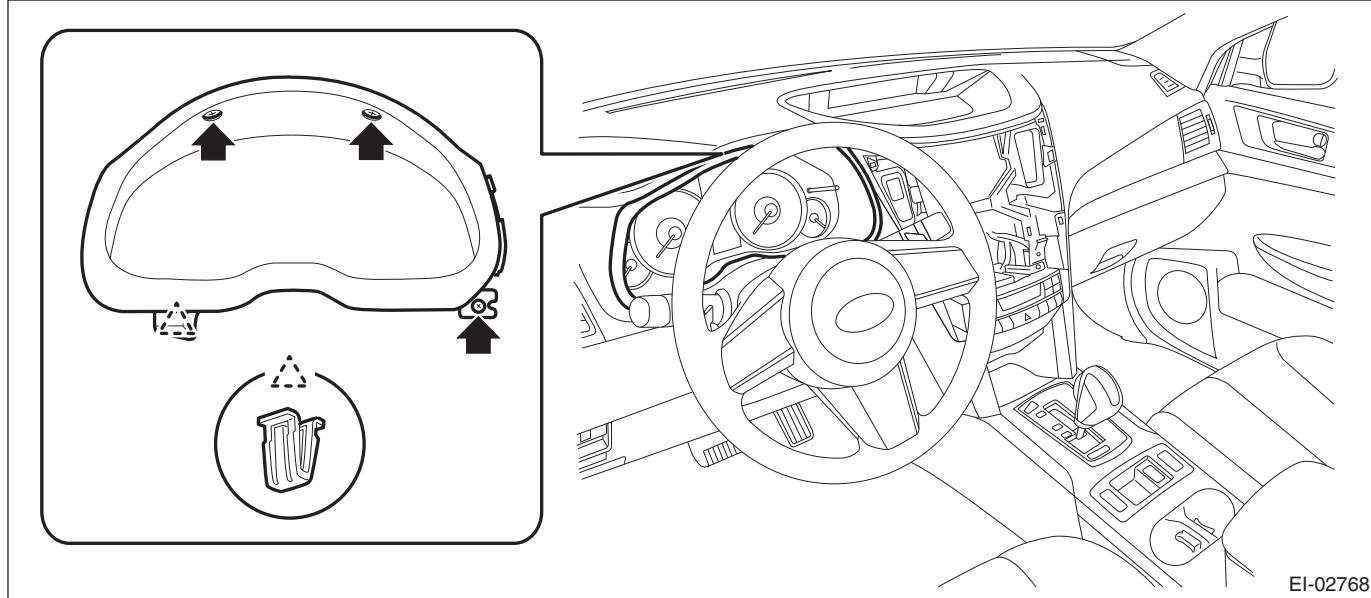
(3) Remove the screws and pull the steering COMPL upper cover toward you.
