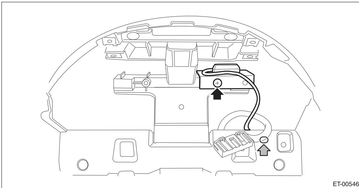
(1) Tie a string to the GPS antenna harness connector on the navigation assembly side.
