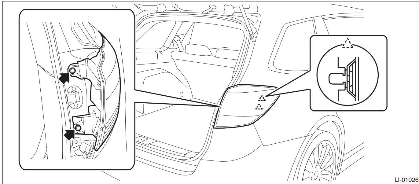
4) Remove the bulb socket and rear turn signal light bulb.
