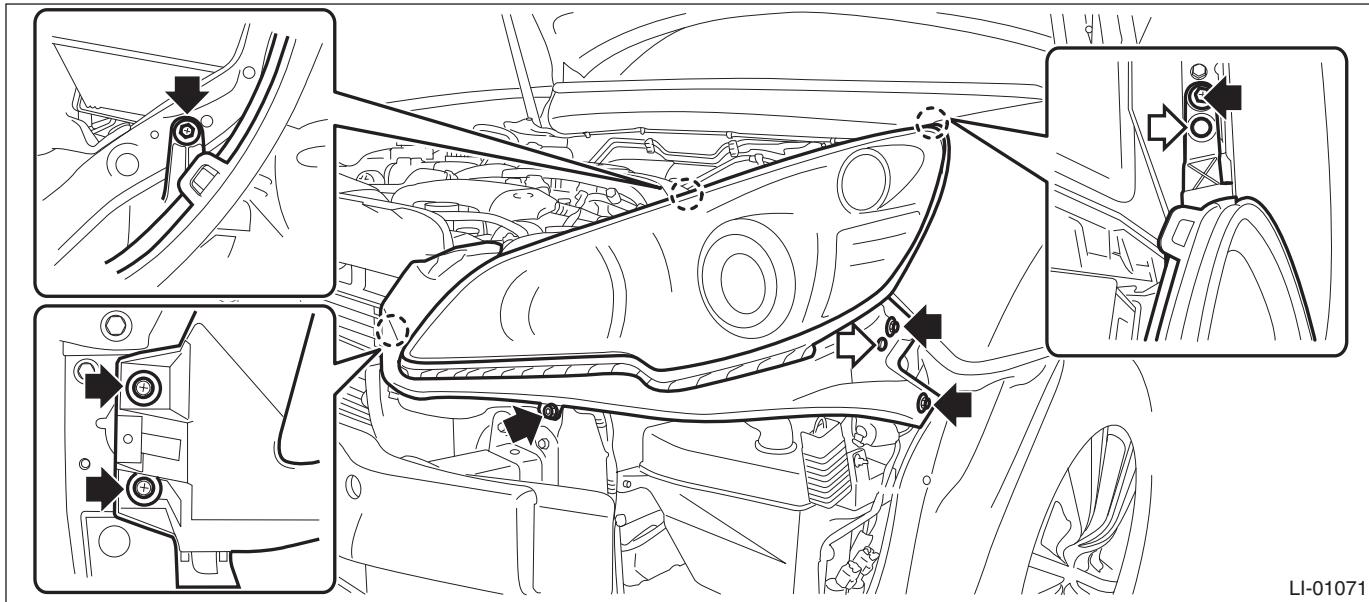
(2) Disconnect the connector and remove the headlight assembly.
