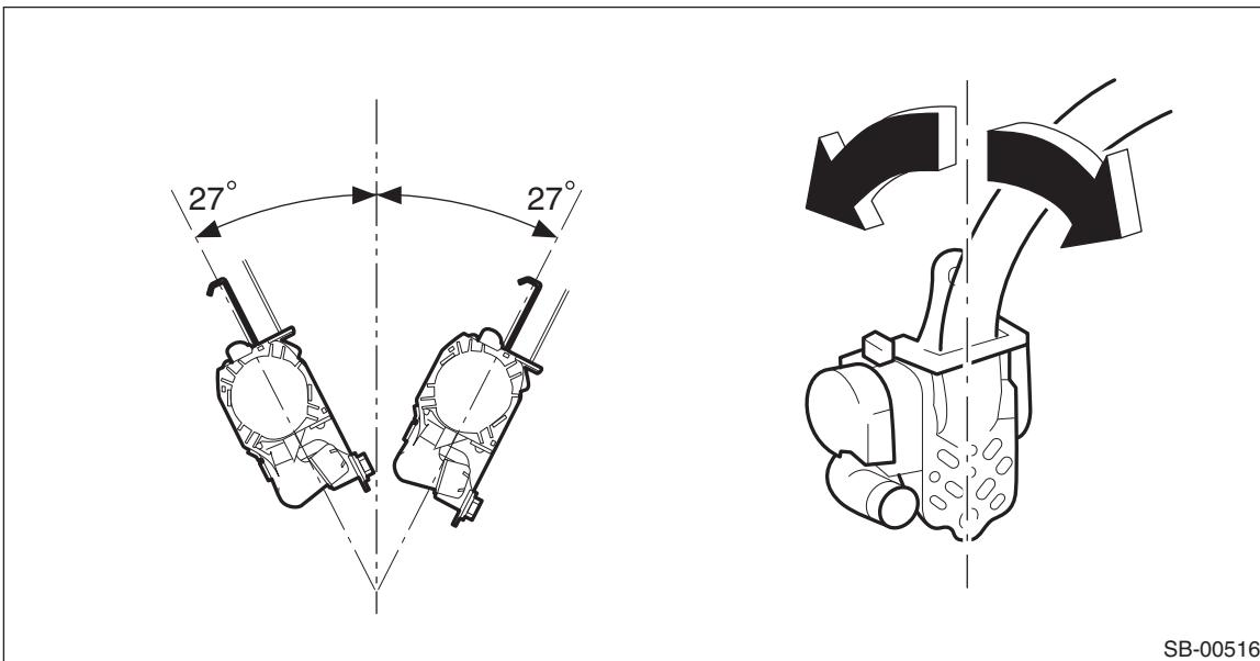
3) If the ELR lock mechanism does not operate correctly, replace the outer belt assembly with a new part.
